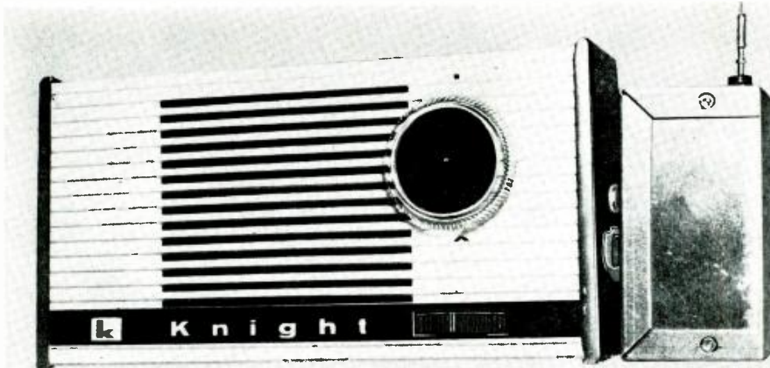
Converter is mounted in small box and is connected to the transistor radio by means of 4-pin connector.
