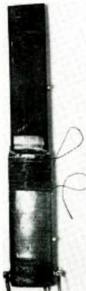
Mixer coil around rod antenna.
