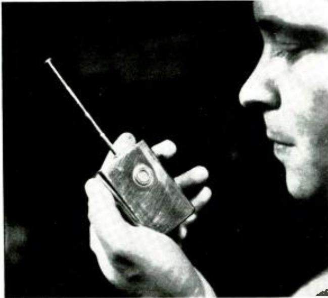
Fig. 1. Miniature transistorized FM transmitter shown in use.
