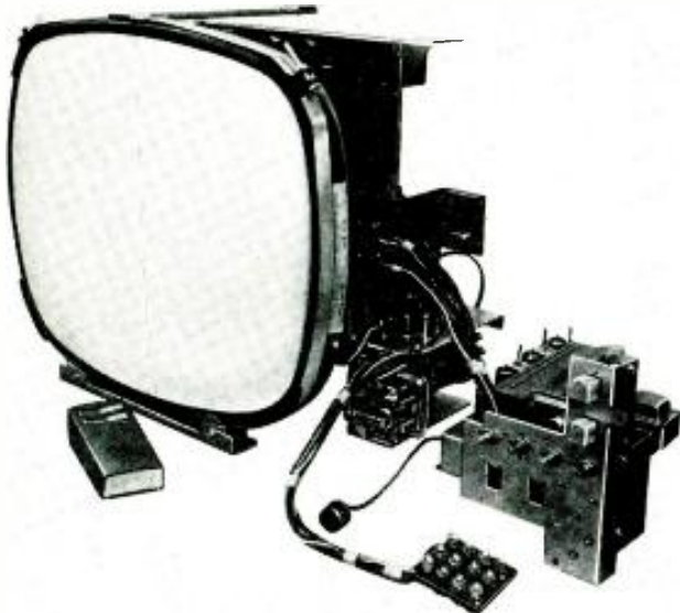
Fig. 4. 12-lamp "computer" panel (lower right) on Packard-Bell mounts behind channel window, lights up chosen channel.
