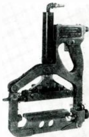
Fig. 12. Two-kw., 40-mc. manual sealer.
