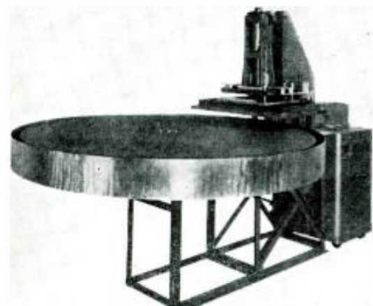
Fig. 11. Wading pool heat sealing press.
