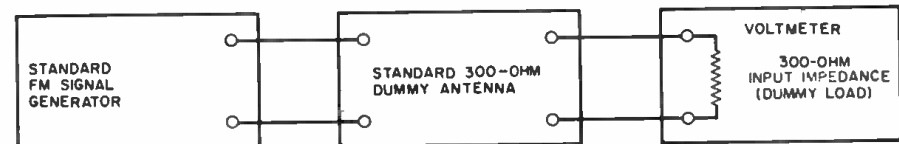
Fig. 3. Method of measurement of input signal intensities and connection method.
