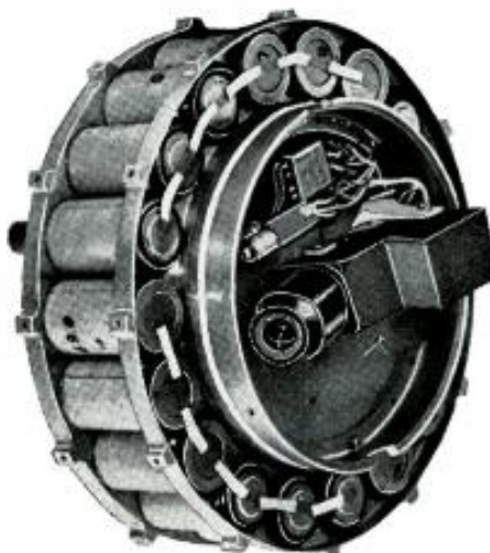
Fig. 17. Series bank of mercury batteries used as power supply in "Pioneer III."
