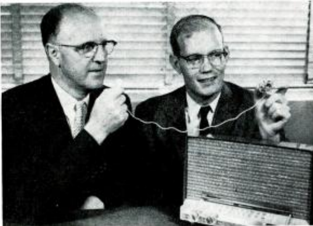
Vest-pocket transmitter, making use of a tunnel diode, and with a range of about one-half mile, is demonstrated by G-E scientists. At left, Dr. Guy Suits, G-E vice-president and director of research, speaks into microphone, while Dr. Jerome Tiemann holds the transmitter. In foreground, ordinary FM receiver picks up signal.
