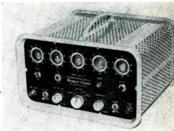
▶ Fig. 7. Device with 5 glow-transfer tubes can count to 100,000. Position of glow in each tube can be read by external digits marked on the panel.
