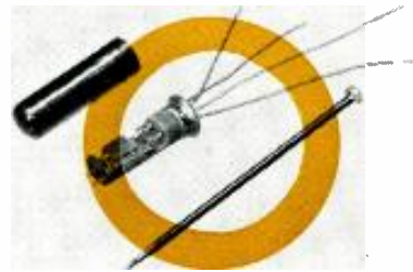
Fig. 4. Germanium resistance thermometer compared in size with common pin.
