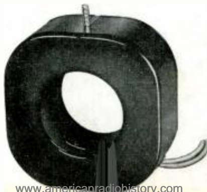
Fig. 8. Typical coil for EM focus. It may be chosen by CRT type number.
