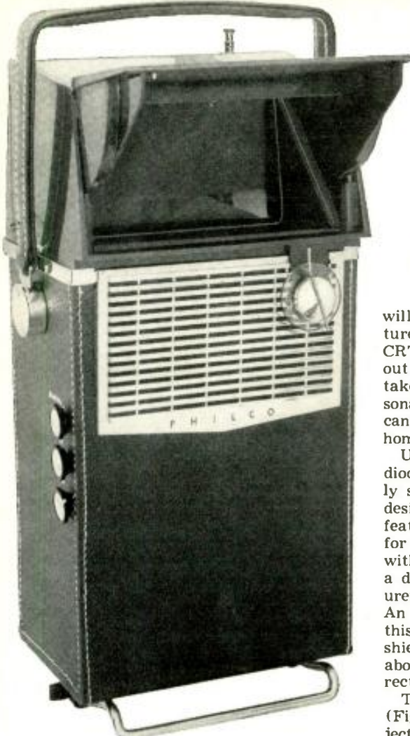
The "Safari" with hood open ready for use. Sloping glass is beam splitter.
