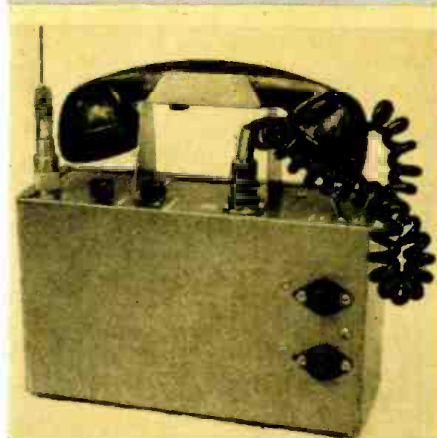
Over-all view of "walkie-talkie" showing power transistors on outside of case.
