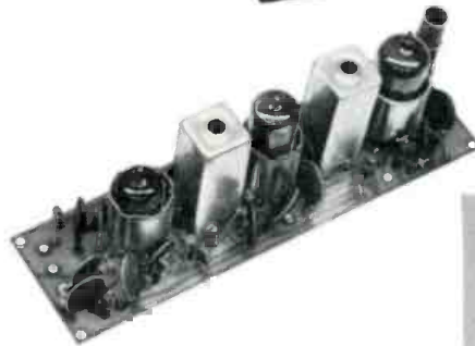
B IF Unit (Printed circuit prewired) Consists of mixer and tunable local oscillator feeding 262 KC IF stage. Includes noise-limiter and squelch circuits. 6AN8 mixer-oscillator, 6BA6 IF amplifier, diode detector, 6AL5 noise-limiter/squelch. Designed to work with units A and C. Makes dual conversion receiver. Shipping weight 2 lbs. $16.00
