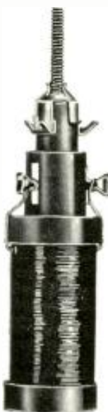
Fig. 4. Standard, adjustable width and linearity coils look like this.
