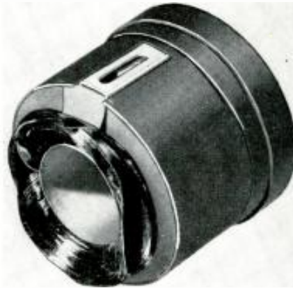
Fig. 6. Typical yoke for 90° or less.
