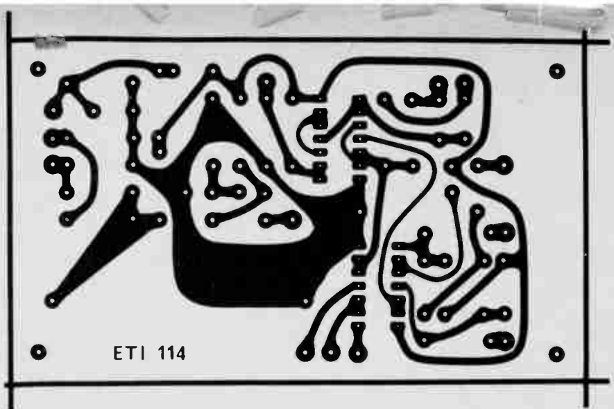
Fig.2. Printed circuit board pattern for the adaptor. (Shown fullsize).
