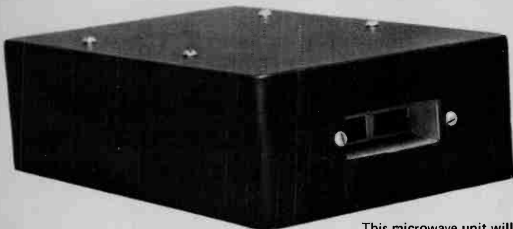
This microwave unit will detect moving objects at ten metres range.
