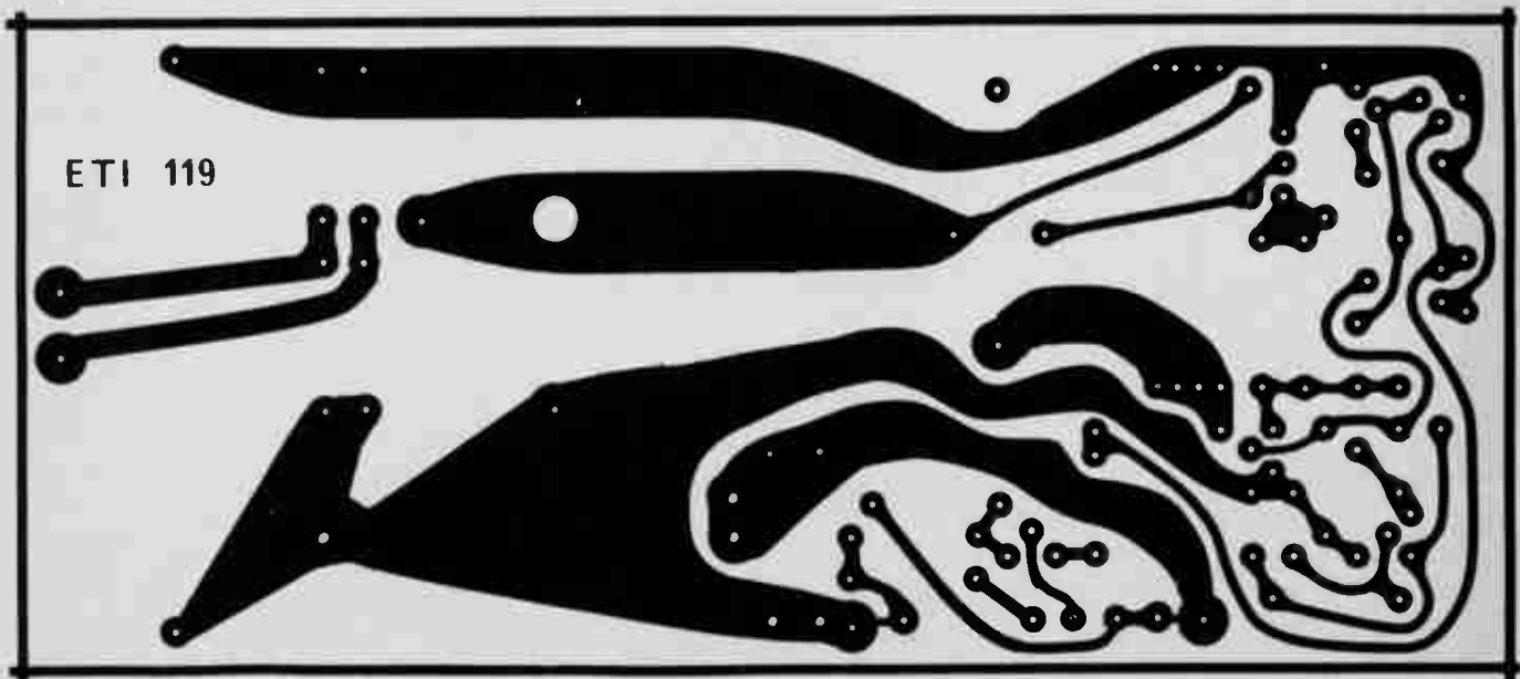
Fig. 5. Printed circuit-board layout. Full size. 178 x 78 mm.
