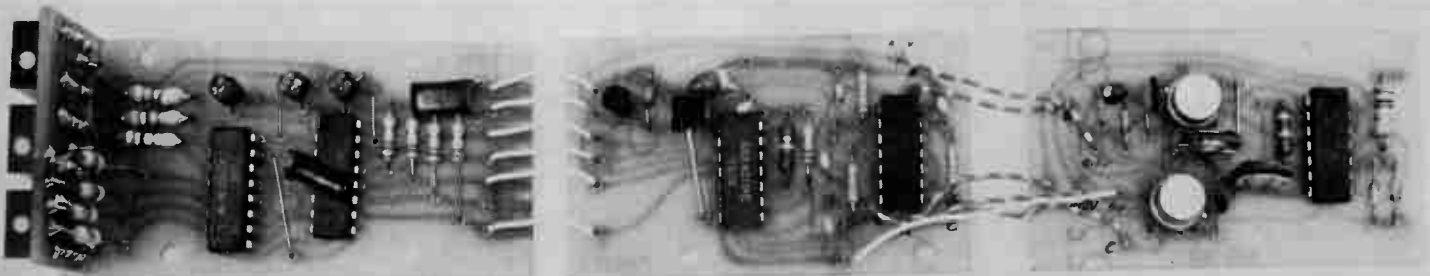
Fig.3. Component overlay of the complete voltmeter.
