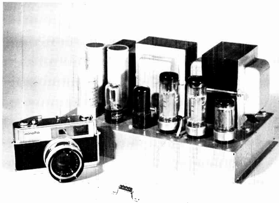
Fig. 5. Dramatically illustrating the rapidly changing nature of electronic techniques, the tiny module has virtually identical performance to the massive unit shown above it. Both are high power audio amplifiers.
