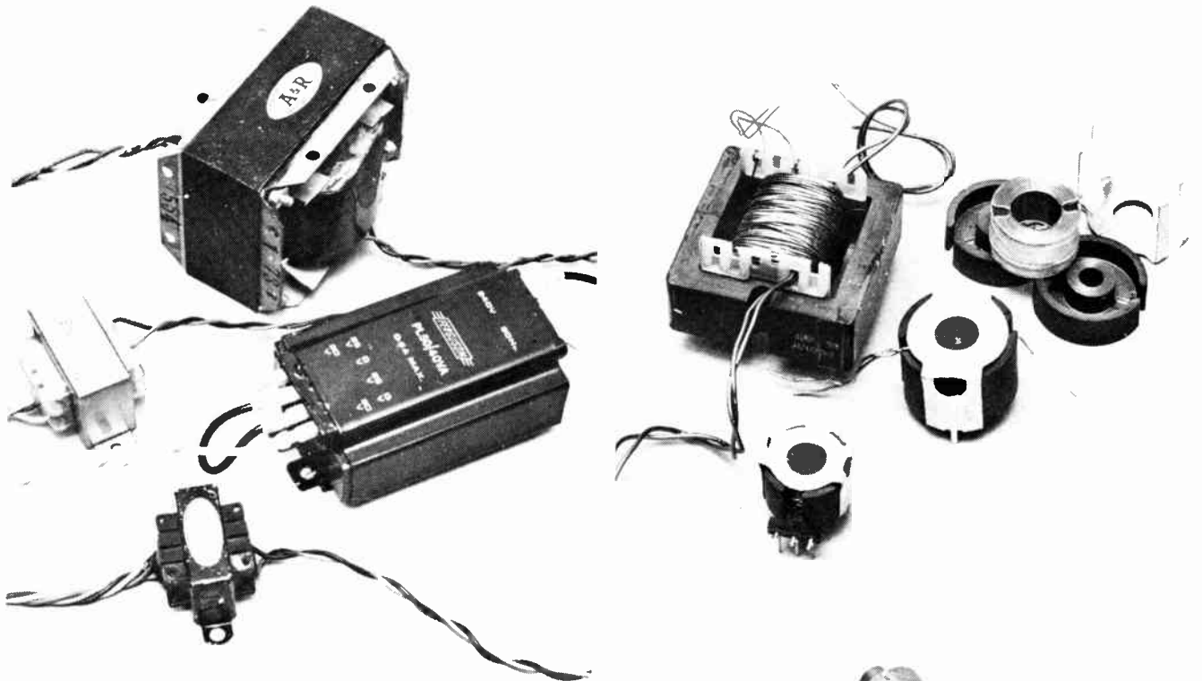
Fig. 3. The design of a transformer depends greatly on the frequency of operation and the amount of power to be handled.
