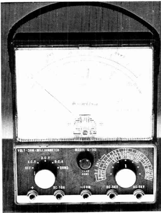
Typical high quality multimeter, note the 'ohms' scale in which zero is at right hand end. Meters that indicate the measurement by a scale and moving pointer are known generically as 'analogue' instruments.
