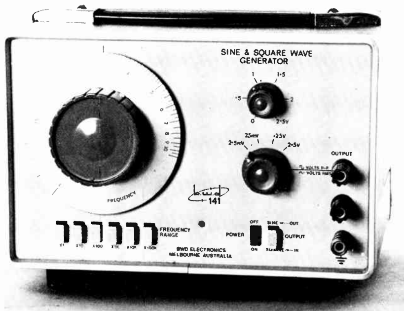
Fig. 2. This audio frequency generator, from BWD, is a medium cost unit that provides adjustable amplitude sine and square waves at frequencies from 1 Hz to 1 MHz.
