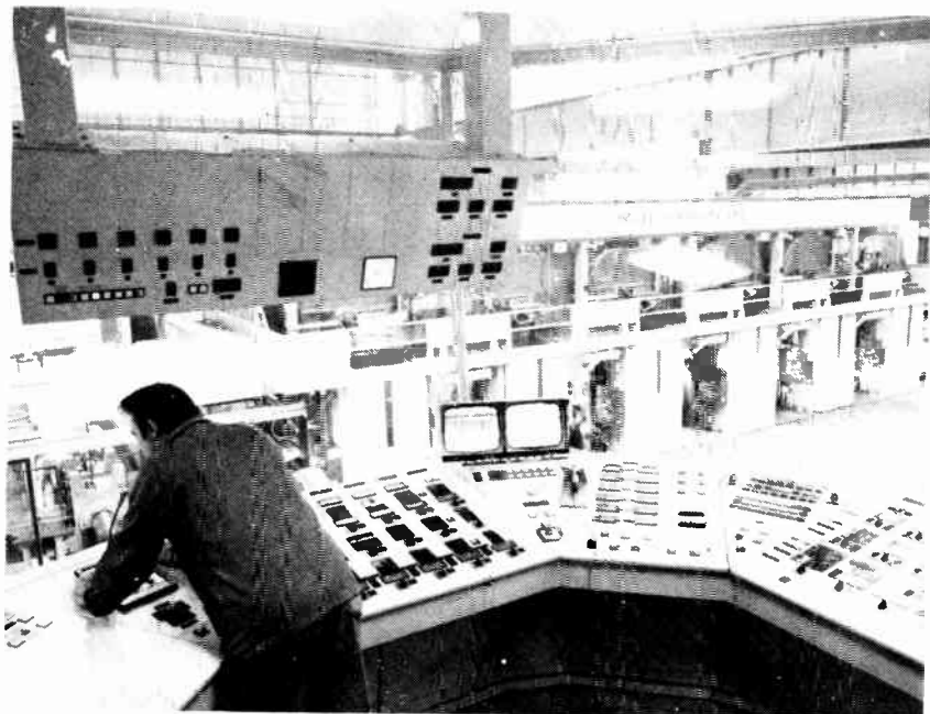
Fig. 7. Signals from many processes may not be in a form suitable for electronic processing. Transducers, are used to make the necessary transformations. Here, information from many different parts of this mammoth steel rolling mill is transduced into electrical form and displayed on this control desk.
