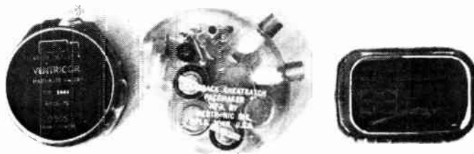
Fig. 5. Three common, fixed-rate implantable pacemakers.
