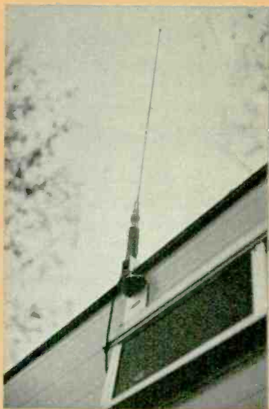
Antenna assembly was mounted on L-shaped bracket eventually located at front right vent window. See text.
