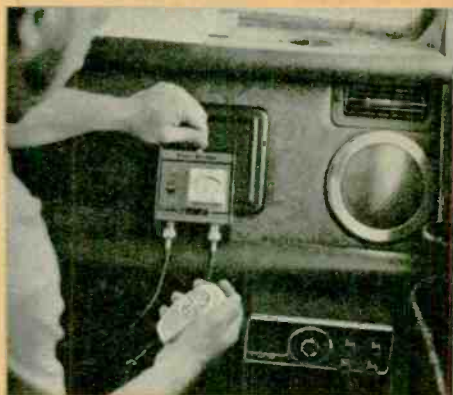
After adjusting SWR meter in forward mode, flip mode switch to reverse position and take reading. Set rig for minimum indicated SWR.
