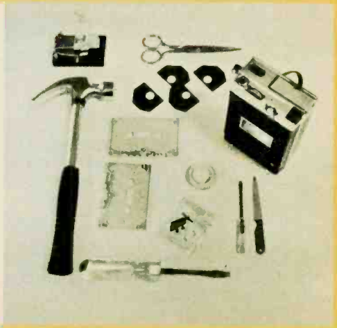
Some basic cassette repair tools. Use a wide-blade screwdriver to break open cassette only in emergency. Recorder comes in handy, too.
