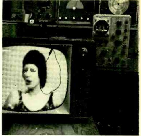
Sweep circuits in TV set generate potent harmonics. Loop of wire in front of set picks up these spiked pulses. Spikes are seen on oscilloscope.
