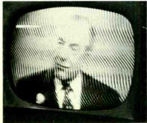
Ted Mack seems to be suffering from beat pattern (from signal close to video frequency) caused by harmonic interference from ham or CB transmitter.
