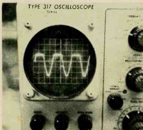
Transistors switch on and off in multivibrator circuit when they reach saturation and cut-off points. Sine wave has flat top when transistor saturates.
