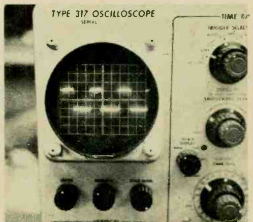
Actual square wave produced by multivibrator. Clipping at top is due to saturation; clipping of bottom portion represents transistor's cut-off point.
