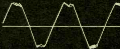
Fig. 6—Distortion produced by overdrive of low-level stages puts waves on the peaks.
