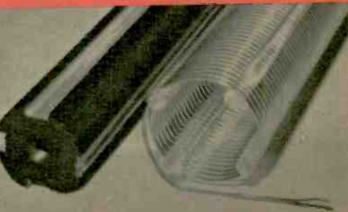
Fig. 8—Photo above shows dowel in which \frac{1}{8} -in. wide x \frac{1}{8} -in. deep channels have been cut to accommodate plastic supports on the coils.
