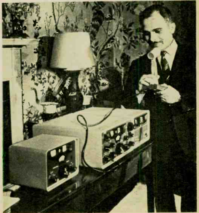
Royal ham station. During his recent visit to the U.S.A., JY1, King Hussein of Jordan, was presented with a Hallicrafters SR-2000 transceiver system at the Blair House in Washington, D.C. Because of the King's on-the-air popularity, he will use the 2-kw rig to cut through the QRM he encounters on the 80-, 40- and 20-meter bands. The system includes the P-2000 AC power supply and the HA20 VFO.
