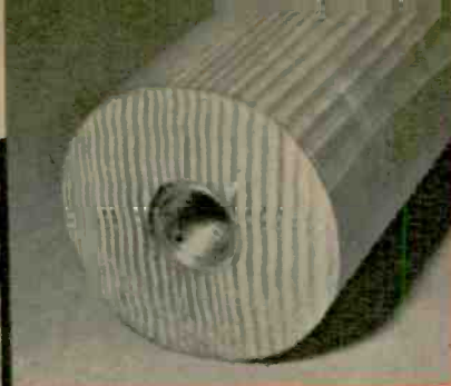
Fig. 7—Prepared nipple is force-fitted in \frac{21}{64} x 2-in.-deep hole drilled in top of the wood-dowel coil support.
