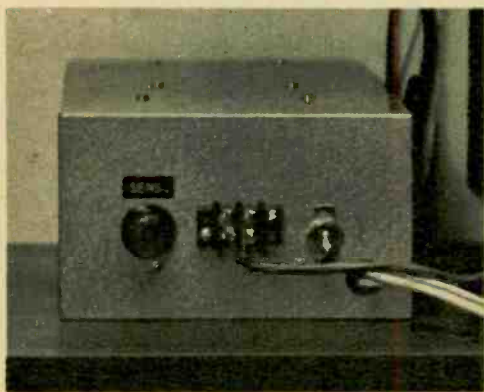
Fig. 1—Control end of color organ which is built in 10 x 6 x 3½-in. Minibox. Wires from speaker go to terminal strip. Lamps plug in other end.
