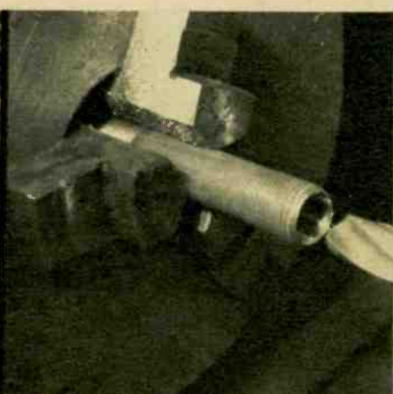
Fig. 5—1/4 NPT pipe nipple must be drilled with 21/64-in. bit prior to threading it with a 3/8-24 tap.
