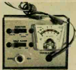
Fig. 4—Troubleshooter supplied with 370 and 169 is 20,000-ohms-per-volt volt-ohmmeter. It is used for check-out.
