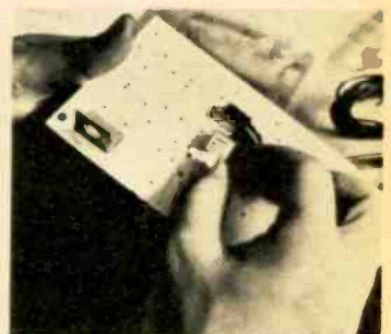
Assembling integrated circuit on a printed circuit board — Circuit is identical to one used in latest IBM System 360 computers. Student is constructing an oscillator combined with a Darlington pair output amplifier.
