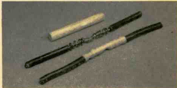
Splice protected by a length of 1/8-in.-dia. tubing. For small applications such as this, a match will supply sufficient heat to cause shrinkage.
