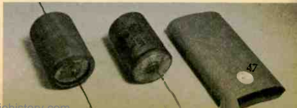
Metal-cased capacitor covered with 1\frac{1}{2} -in. dia. tubing. In crowded circuits it's good idea to cover case to prevent other parts from shorting to it.
