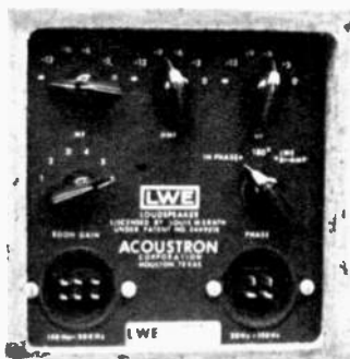
Woofer, lower- and upper-mid-range, tweeter, room-gain controls.
