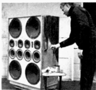
Applying stain finish to cabinet. We applied wax after stain dried.
