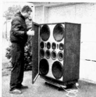
Because speakers are recessed, grille-cloth frame mounts flush.
