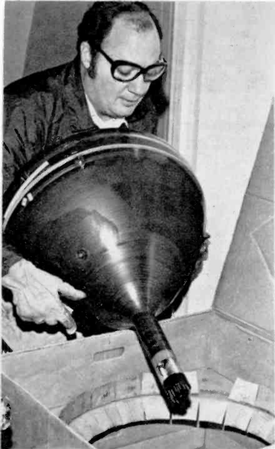
Band is attached to new tube. Be careful to see that the hole in the band is between glass ridges. The ridges indicate the top of the round tube.
