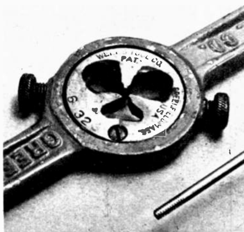
Fig. 3—The dia. of CB whip 24 in. from top is 0.138 in.—the dia. of 6-32 screw. Thread whip end using 6-32 die which is shown above in stock.
