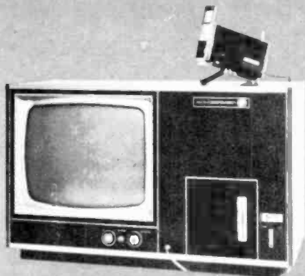
Fig. 2—Avco's Cartrivision. Admiral will market it for $900. You can play shows, record off the air or tape your own home TV shows.
