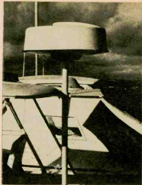
Radar antennas go in circles. At left is scanner of Decca's new Super 101 radar, at the right is radome of Raytheon's 2900. Both connect to T/R unit via coaxial cable; usual microwave plumbing is absent.
