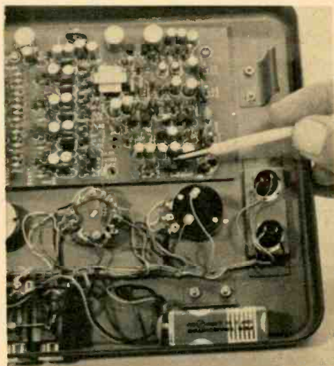
Fig. 5—Tool touches "bd pit" (bass-drum pitch) pot in Knight-Kit. To find pots in other units, position units as shown and locate as in the text.
