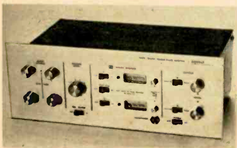
Noise Reduction Center by Advent is first component to use Dolby System for home tape recording. Unit goes between amplifier and recorder.
