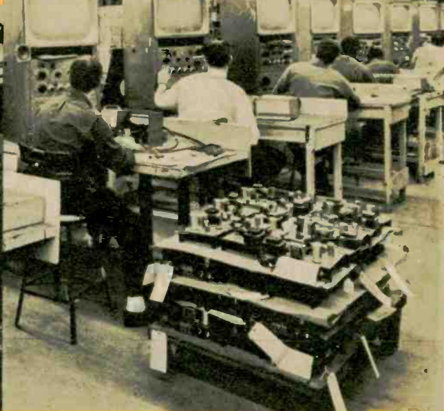
Technicians on inspection line in large plant use large-screen scopes to make final tests on amplifiers.
