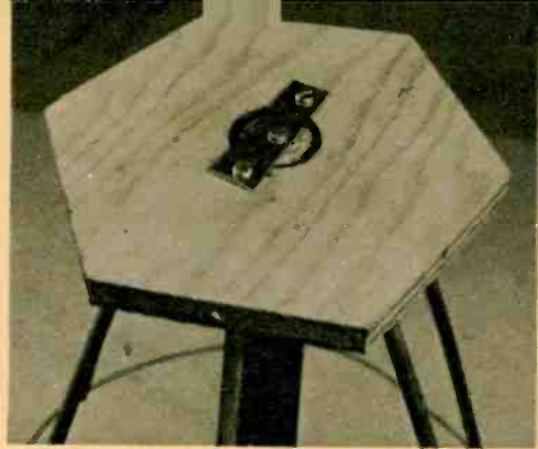
Fig. 3—Back of hub. Force fit short lengths of 1½-in.-dia. dowels in each end of boom. Attach hubs firmly to boom with 3-in.-long pieces of metal.
