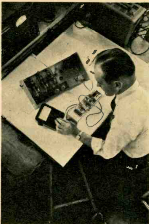
Technician in engineering lab at Bogen Communications checks out relays for a paging system.
