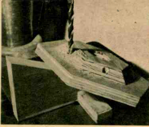
Fig. 2—To drill the angled holes for the 2-meter-antenna dowels, use a wedge with a 20° angle. Holes should be drilled to ½-in. depth.
