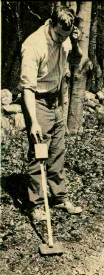
Birch handle, left, is about 3 ft. long and folds in half for storage. Center photo shows electronics. Outputs of two FET oscillators go to mixer which is followed by two audio stages. Search head, right, is glass-epoxy board that is used without cover. A coil is etched on top side, a shield is etched on other.
