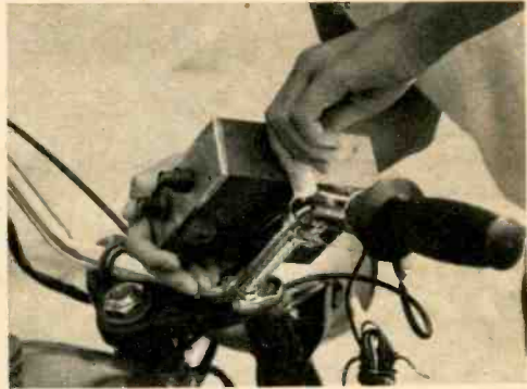
Fig. 2—Install the transceiver in the gimbal using star washers between the bracket and transceiver to prevent mounting screws from loosening.
