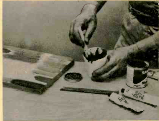
Fig. 2—It's easy to match colors when you use oils. All you have to do is dissolve the color in turpentine and then compare it with the sample.
