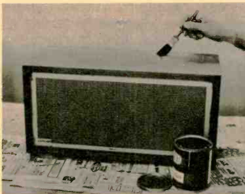
Fig. 5—After the cabinet has been stained and wiped with a soft cloth, apply a coat of clear sealer to the surfaces with a small paint brush.
