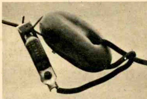
Fig. 7—To switch bands, sections of legs must be added or removed. Quick and easy way is with porcelain strain insulators and alligator clips.
