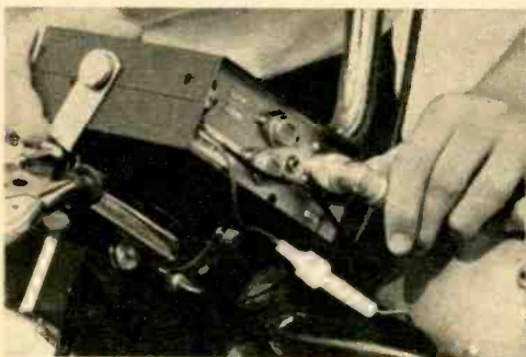
Fig. 6—Bring wires through opening in center of fork, make loop and connect to transceiver. Put connectors on battery wires so rig can be removed.
