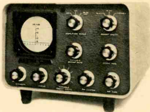
(5) Scanalyzer (Heathkit Model SB-620) is panoramic adaptor that displays a 150-500 kc segment of a band. It also displays transmitter's output.
