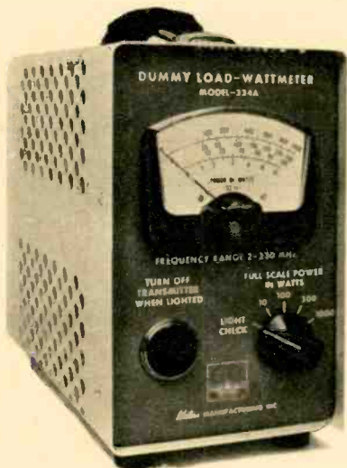
(3) Dummy Load/Wattmeter (Waters Model 334A) measures transmitter's output into 52-ohm dummy load up to 1 kw. Its frequency range is 2-230 mc.
