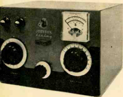
(2) Matchbox (E. F. Johnson, Viking) matches transmitter's output into almost any kind of antenna. This model (250-23-3) handles up to 275 watts.
