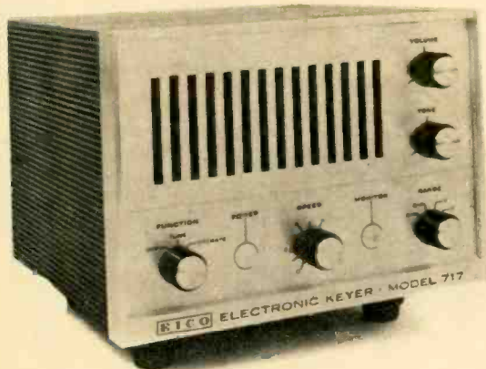
(6) Keyer (Eico Model 717) produces perfect dot-dash-space ratios at 3-75 wpm speed. Built-in speaker lets you hear your fist while you send.
