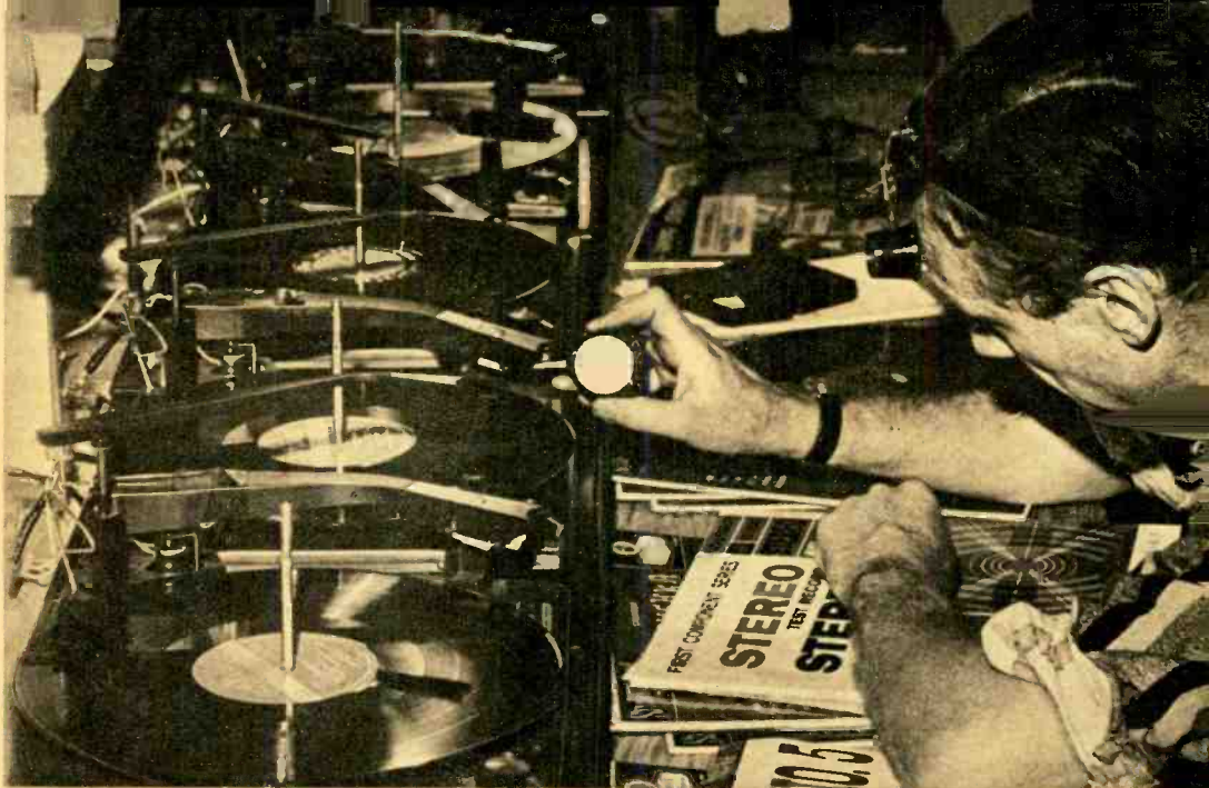
Exhaustive wear tests by EI used a battery of modified changers with various cartridges to play small portion of records over 1,000 times in some cases. Here stylus tracking force is being double-checked.
