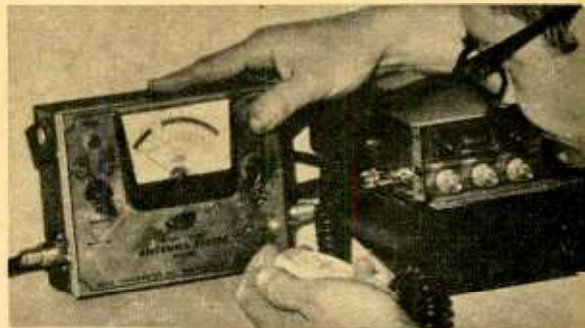
Fig. 3—After installation of antenna and coax, connect an in-line power/SWR meter between coax and transceiver to measure SWR and output power.
