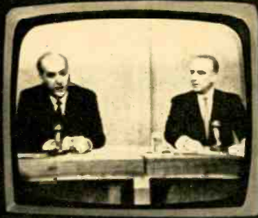
Fig. 3—Photo at right is of TV set operated on 117 VAC. Photo at left is of TV set operated from power pack. Note that picture is smaller in height and width (studio camera change further reduced size of men). Loss is due to lower B+ voltages caused by square-wave input power.
