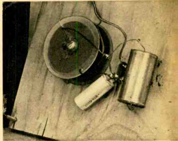
Fig. 3—Contour network parts should be attached to back panel with epoxy cement so they won't rattle. Do not use an iron screw to hold the coil.
