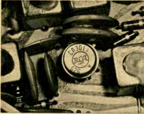
Several integrated circuits may be used in a modern CB transceiver—in IF strip, as AF amplifier or (as in the case of the IC at the center of this photo) as RF amplifier in noise-silencer circuit.
