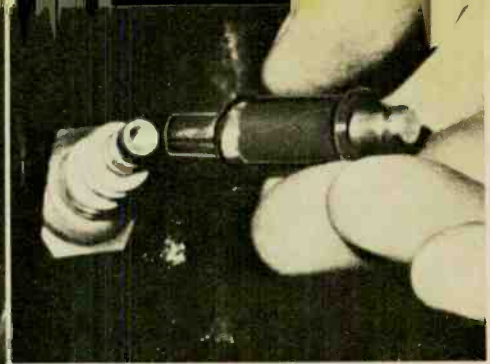
Fig. 3—Top. If your car does not have resistance plugs or resistance-wire plug cables, a carbon noise suppressor must be added at each plug. Left. All primary ignition leads including the feed to the high-voltage coil should be filtered with coax shielded capacitor. Make certain all of the connections are good and tight.
