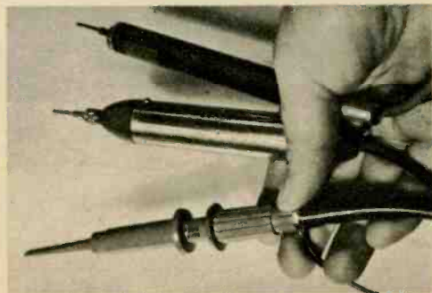
Fig. 5—Attenuator probe (bottom) prevents circuits from being loaded. Middle probe is for measuring RF voltage. Top probe is RF demodulator.
