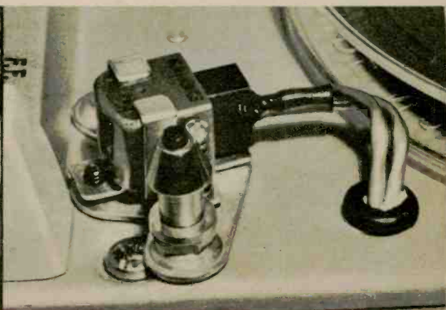
Fig. 3—Completed deck installation. Connecting block attaches cables to head. Adhesive in the grommet keeps the cables firmly in place.
