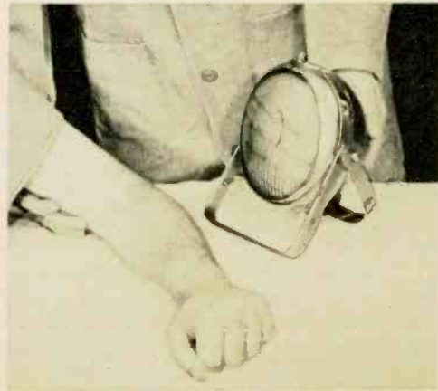
Depolaray consists primarily of AC electromagnet rigged to cause buzzing on lens. Instructions suggest adjusting the sound to please patients.
