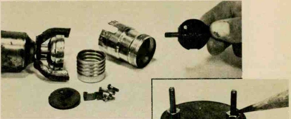
Fig. 3—If rivets were used to hold the socket together, drill them out. Discard switch assembly (in hand) but save all other parts. Cut short the screw (No. 2 or No. 3, ½ in. long) indicated by pencil—the one opposite the center-contact slot.
