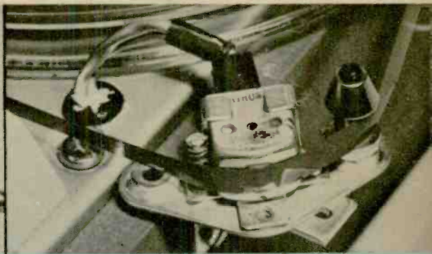
Fig. 6—Completed outboard installation. Again, a Nortronics connector is used to attach cables to head. Don't forget adhesive in the grommet.
