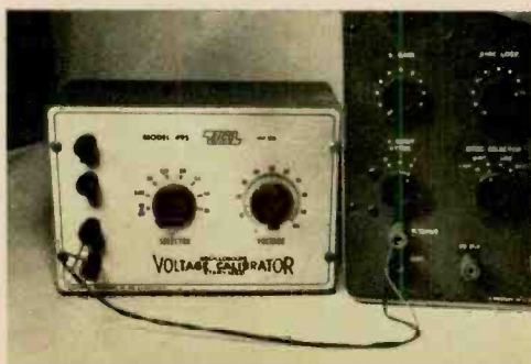
Fig. 7—Voltage calibrator, an external accessory, provides an accurate reference trace for measuring the amplitude of the signal being displayed.
