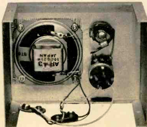
Fig. 2—Cabinet before installation of board. Connect wire from ground buss on circuit board to solder lug on one of speaker's mounting screws.
