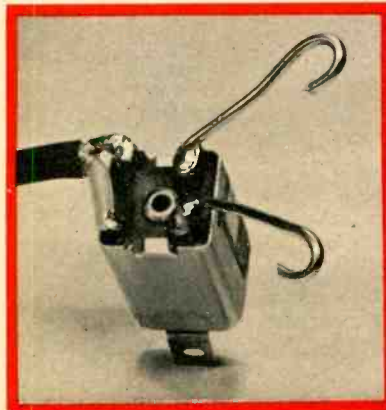
Solder heavy wires, spread to fit antenna terminals, on transformer's 300-ohm lugs. Keep coax's shield short.
