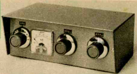
Front view of transmitter, above. Left control is VFO, meter indicates final's collector current, center control is final's collector tuning, right control is loading. At the left is a photo of the rear of the transmitter.
