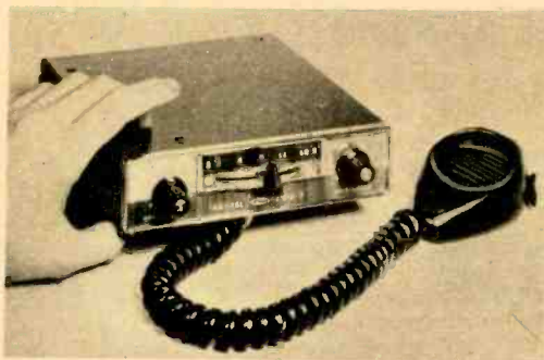
First CB set specifically designed for the proposed HELP service, Raytheon's TWR-7 deliberately is on the simple side and largely goof-proof.
