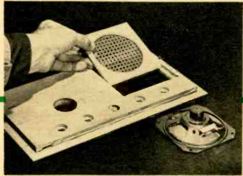
Fig. 5—Details and dimensions for a 1/2-in. walnut-veneer cabinet. Speaker is attached to a piece of 3/8-in.-thick plywood which is mounted in front panel. Tie rope around the cabinet to hold joints together while the glue dries.
