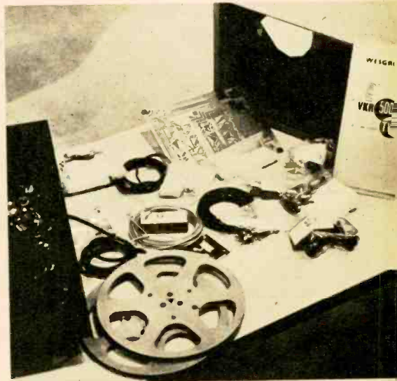
Kit consists of basic tape-transport mechanism and necessary record and replay electronics. Most components mount on single printed-circuit board.
