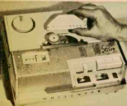
Cover must be removed to permit access to most heads. Step usually requires removal of a few screws.
