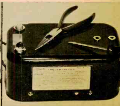
Tools always should be demagnetized with a bulk tape eraser before bringing them near tape heads.
