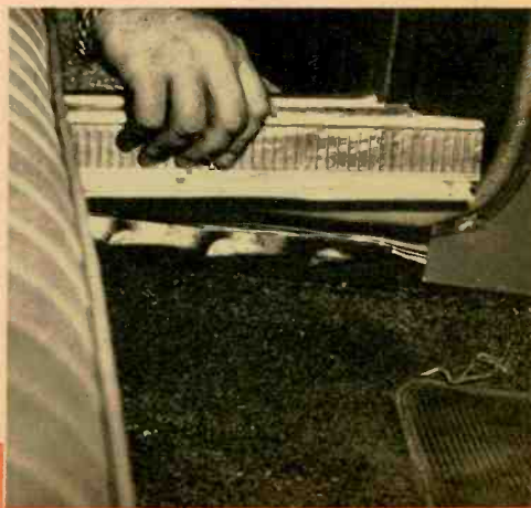
Wiring channel can be exposed by removing front and rear door kick-plates. If present, channel offers ideal way to hide coax transmission line.
