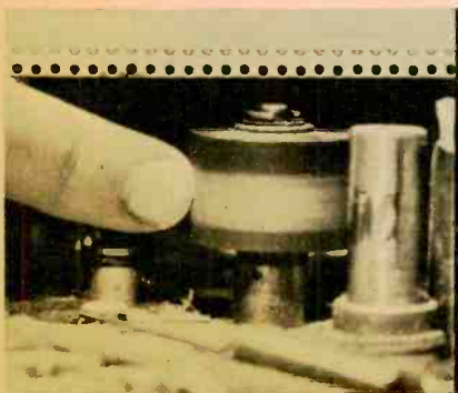
Oxide flake-off on capstan pinch roller shows cleaning is called for. A Q-tip again is required.
