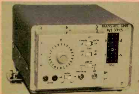
International Crystal 750-HB2 comes equipped for instant troubleshooting. Voltages and currents are sampled, then fed to meter jacks at lower left.
