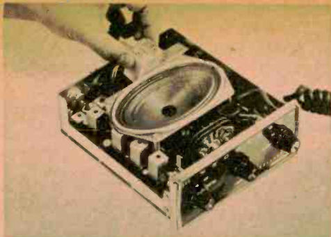
Johnson Messenger III's small size belies its 5-watt rating. Note sealed, computer-grade changeover relay (in hand) and top-up speaker mounting.
