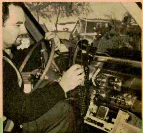
Microphone can be replaced with handset for maximum convenience. Lifting handset from cradle cuts speaker, feeds audio into handset earpiece.
