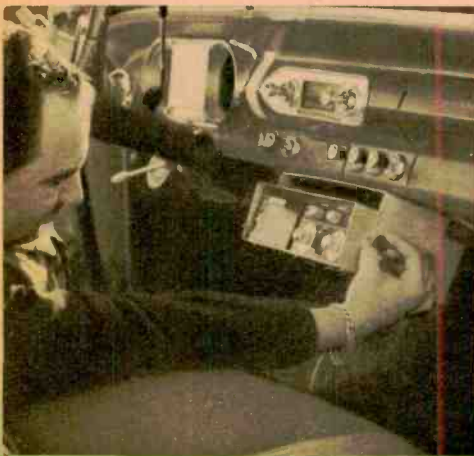
Transceiver must fit snugly in bracket if unnecessary vibration is to be avoided. Lockwashers under thumbnuts often make for increased rigidity.
