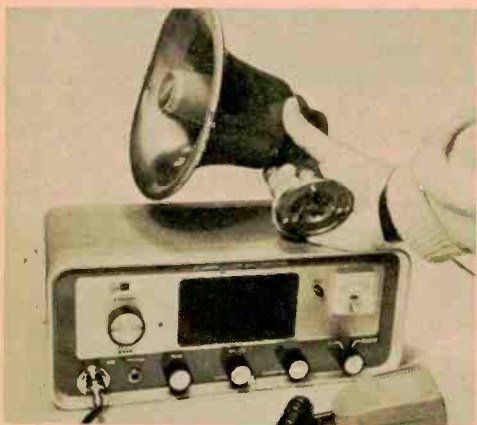
Knight KN-2565 numbers among transceivers with provision for public address. Bull-horn speaker (in hand) mounts on car or other nearby support.
