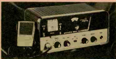
Regency Romper sports new twist in frequency syntheses. Single crystal plugs into socket below meter, serves both transmit and receive circuits.
