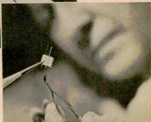
Surgical-type preparation is given to small sliver of ceramic material that contains ten solid-state diodes. Scissors are kind used in eye operations; note the filmy surgical gloves.
