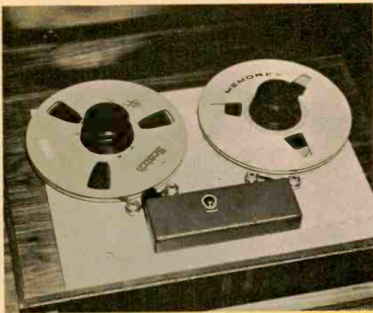
Fairchild's proposed entry into home TV recorder field. Though machine can use standard 1/4-in. tape, instrumentation tape works much better. Such tape produces less head wear, keeps heads cleaner.
