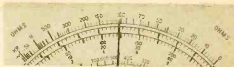
Fig. 2—Mid-scale resistance of this VOM's ohmmeter scale is 100 ohms. If battery is 1.5 V, when range switch is at R \times 1 current through shorted probes is 1.5 V divided by 100 ohms, or 15 ma.
