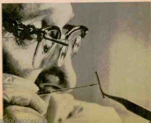
Using a miniature scalpel, a scientist trims the gaps in an ionic switch. Device becomes a conductor if sufficient voltage is applied to enable it to ionize gas in its envelope.
