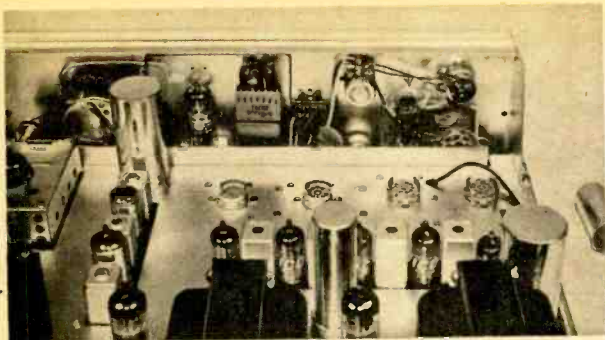
Rear view of 2536. Front-end is at extreme left, multiplex adaptor is at right of it. Preamp tubes have been removed from sockets, IF strip is below them. A metal cover fits over the control panel.
