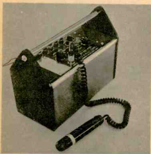
Audio amplifier boosts signal from mike, feeds it into loop of wire which surrounds pool completely.
