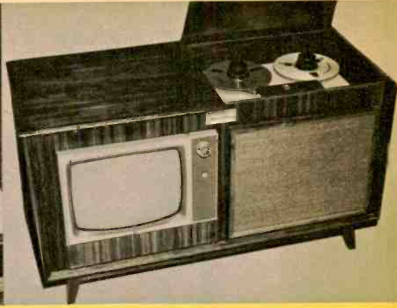
Fairchild's proposed entry into home TV recorder field. Though machine can use standard 1/4-in. tape, instrumentation tape works much better. Such tape produces less head wear, keeps heads cleaner.
