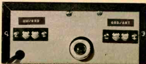
Rear view of preamp. VI sticks out of 1½-inch-diameter hole in center. Connect receiver to terminal strip at left. Connect antenna at the right.
