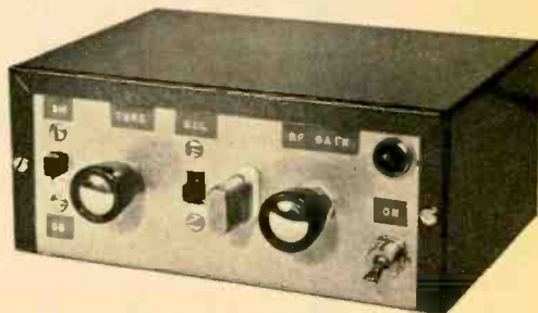
Preamp fits in 3x5x7-inch Minibox. Attach receiver and antenna to it permanently. Switch at left connects antenna to receiver directly or through preamp.
