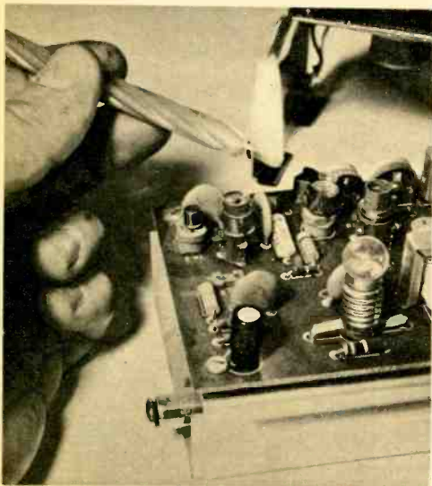
Add a little wax, and loose tuning slugs freeze in position. See text for tips on how it's done.
