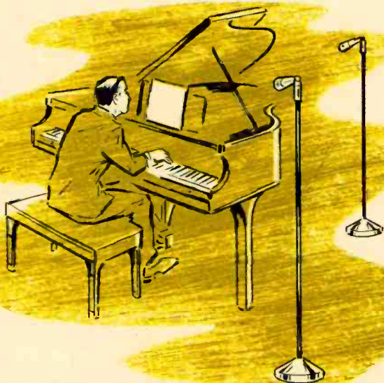
Solo piano tapes well with mikes located about 8 ft. from longitudinal center of the instrument. Best sound seems to result when one mike is placed at end of keyboard, other mike at front or rear.
