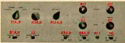
Fig. 8—Front panel is a 14½x4¾x¼-inch-thick piece of aluminum. After drilling, have panel sandblasted, and then letter it with transfer type.
