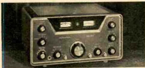
The SX-117 triple-conversion receiver tunes SSB, CW, AM with first and third oscillators crystal-controlled. Includes crystals, variable 3-step selectivity control and BFO. $379.95. Hallicrafters Co., Chicago, Ill.
