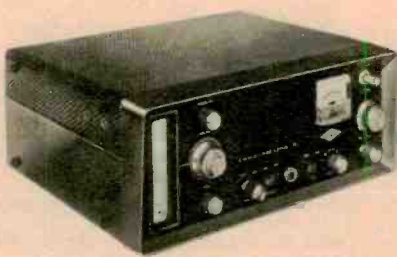
The Communicator IV triple-conversion AM transceiver comes in 2- and 6-meter models for mobile or fixed use. Built-in speaker. $389.95. Gonset, Burbank, Calif.
