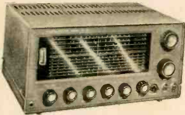
Lafayette's HE-30 receiver tunes 80-10 meters with full coverage from 550 kc to 30 mc. Wired, $99.95; semi-kit (KT-320), $79.95. Lafayette Radio, Syosset, N. Y.
