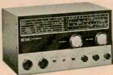
The Knight R-55 receives 530 kc to 36 mc plus 47-54 mc. Tunes 80- through 6-meter ham bands. Built-in speaker, power supply. Kit, $59.95. Allied Radio, Chicago, Ill.
