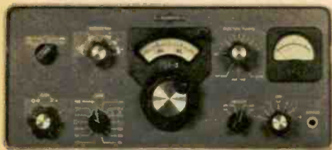
Collins' 755-3 is an SSB/CW/RTTY ham receiver. Bands are covered in spread-out 200-kc segments. Crystal filter for CW. $680. Collins Radio, Cedar Rapids, Iowa.
