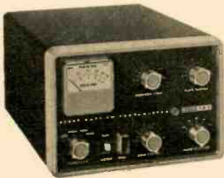
A crystal-controlled CW-only transmitter for the beginner is the EICO 723. Input is 60 watts peak. Kit, $49.95; wired, $79.95. EICO, Long Island City, N. Y.
