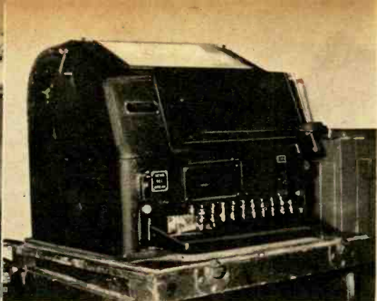
Teletype machines used by RTTYers are models which have been discontinued by the Teletype Corp., such as the Nos. 26 and 15 pictured above. A few hams have purchased surplus Kleinschmidt teleprinters.
