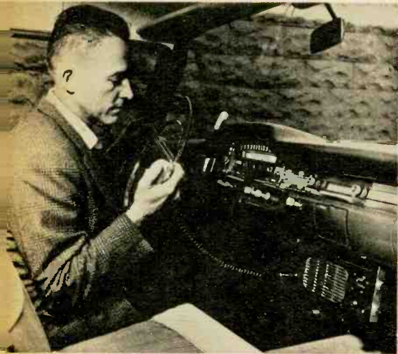
Mason shows off one of his SSB CB units mounted for mobile operation. Set draws about 42 watts.
