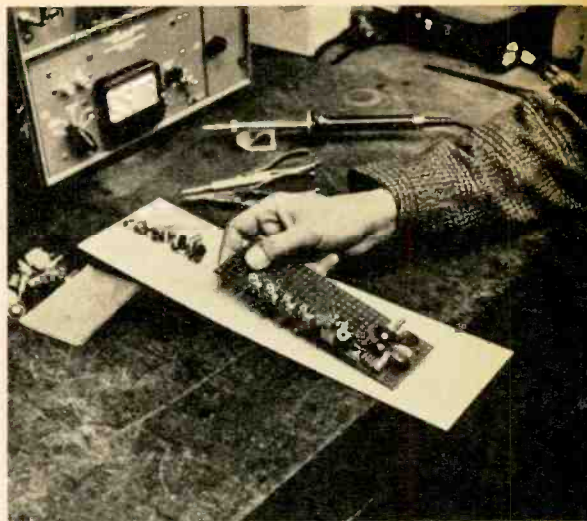
Transistorized version of transceiver is under construction; whole circuit will fit on board.
