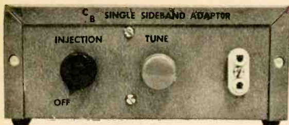
Transmitting crystal plugs into socket at the right. Both the injection and tuning knobs are carefully adjusted for the clearest audio signal from an SSB transmission.
