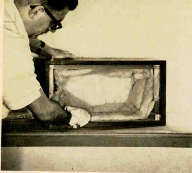
The author's prototype had front panel removable. Here the cabinet is being lined with a layer of glass wool.
