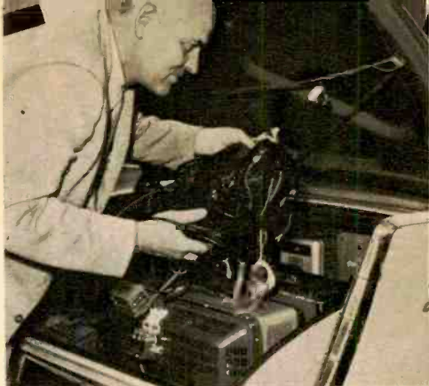
Chock-full trunk includes cables for setting up field antennas and inverter to supply 117 volts.
