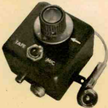
Fig. 2—Signal Conditioner, built in metal box. Interconnects a tape recorder and transmitter.
