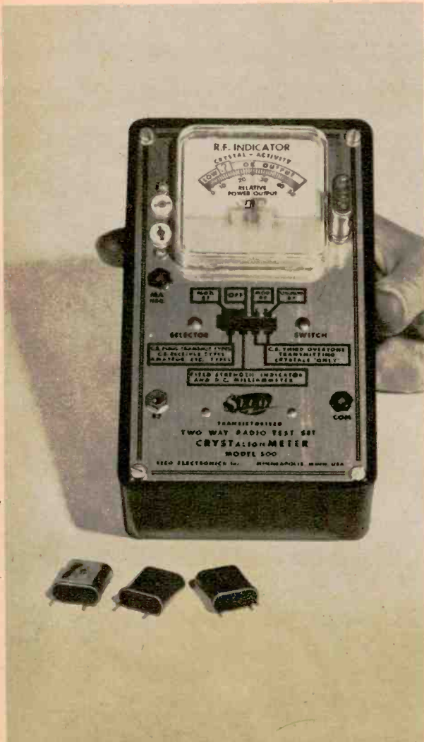
Multi-purpose CB test set by Seco performs a wide variety of tests, including crystal activity checks.
