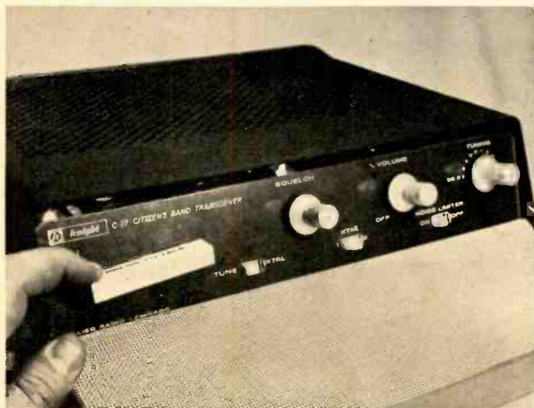
Large press-to-talk bar is handy feature of the Allied Knight-Kit C-27 transceiver; kit costs $79.95.
