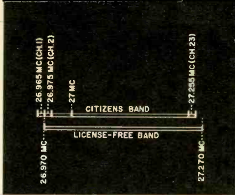
The License-Free and Citizens Bands are not the same but the two do overlap on most frequencies.
