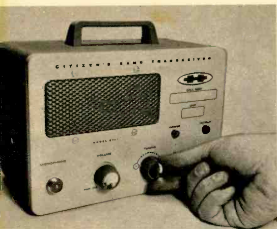
Superregen tuning knob gives approximate channel markings. Heathkit CB-1 (kit) sells for $42.95.
