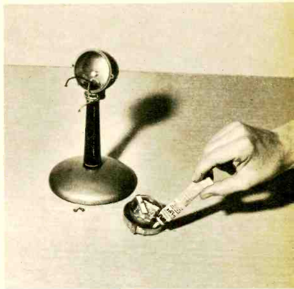
Position cartridge in case and glue shock mounts in place. New shocks may be made of excess rubber.
