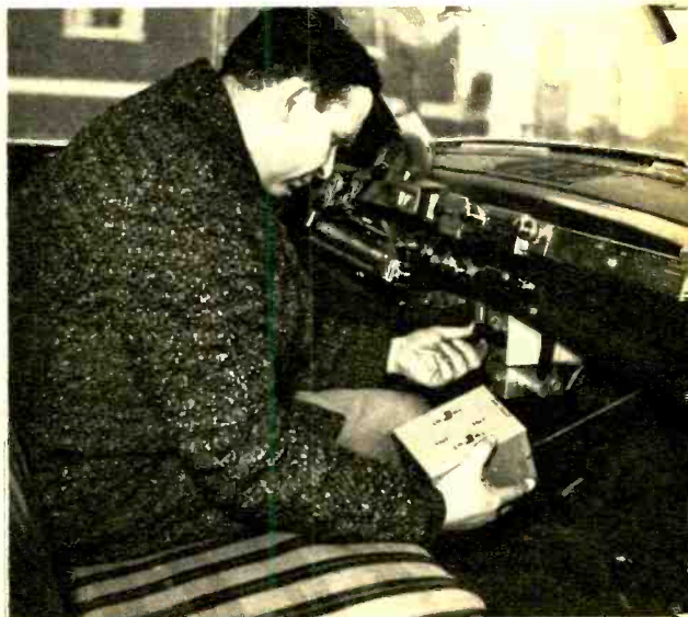
Most parts are mounted on perforated board which is installed in cabinet using small brackets.
