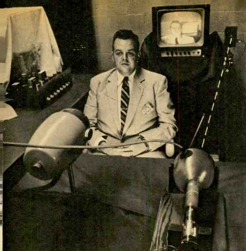
Experimental Westinghouse apparatus transmits video (picture) information on narrow beam of modulated ultraviolet light. Left foreground is camera, right background is transmitter. Photomultiplier, which feeds signal to TV set, is in right background. The broken white line represents invisible UV beam.
