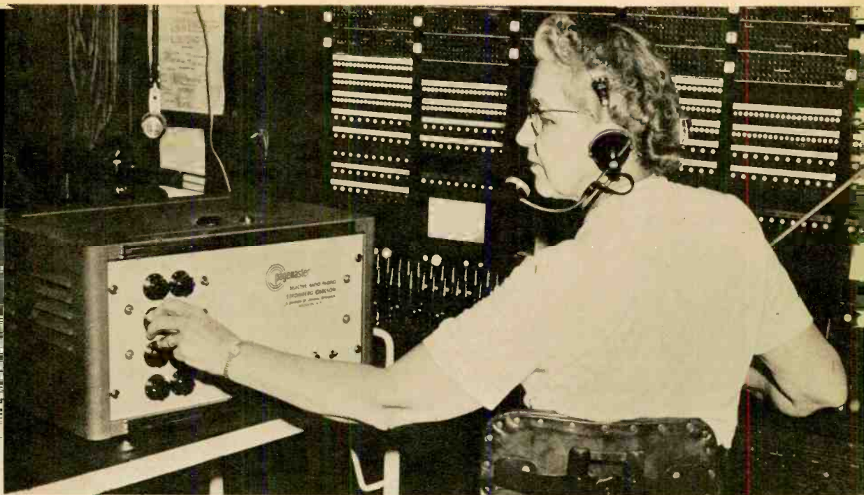
Telephone answering service uses radio paging system on four frequencies. A radio paging system in Hawaii is often received in the continental U.S.
