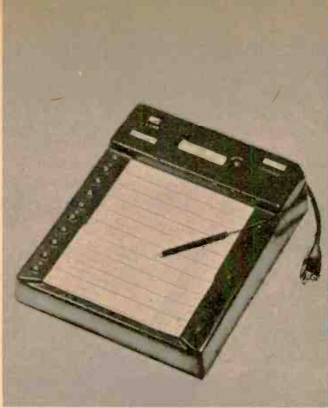
Questions on Astra electro-mechanical Auto-score are answered by putting probe in holes and lights respond; it tallies errors and time.
