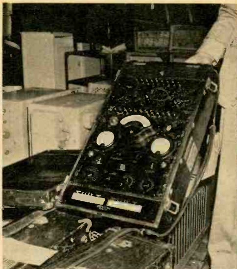
Elaborate portable tube checker is complete with cover at the left and a carrying strap. Other surplus checkers appear in foreground.
