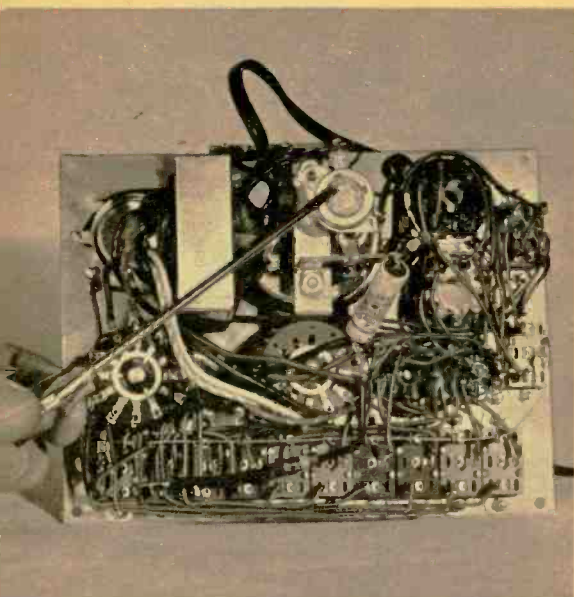
Screwdriver indicates calibration pot. Extreme care was necessary in soldering sockets. Schematic shows circuit for emission test made at low voltage with grids and plate tied together.
