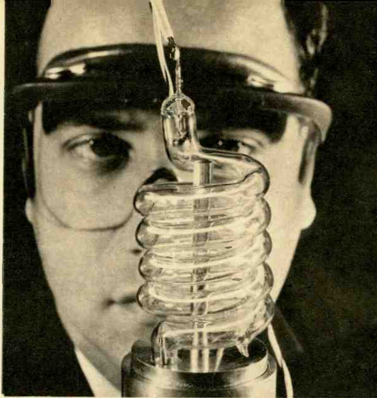
Helical neon tube-like light exciter surrounds rod of synthetic ruby. This is the heart of the Laser light amplifier. No magnetic field is necessary.
