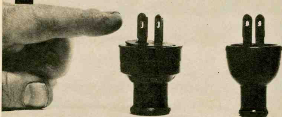
Attachment plug at left is hard-to-get two-prong polarized type. Finger points to the wider of the two prongs; this is the "ground" side of the circuit. Polarized plug can go into circuit only one way. Center plug is ordinary type, can be inserted two ways. At right is the new type three-prong polarized safety plug. The one longer, thinner prong is for ground.
