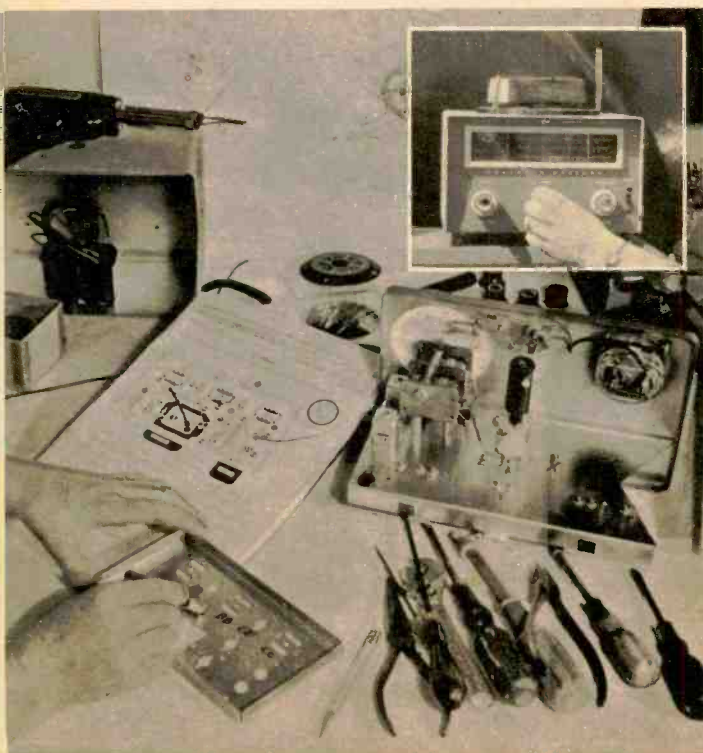
Heathkit DF-3 ($99.95) is 9-transistor radio direction finder kit for aeronautical, broadcast and marine bands.
