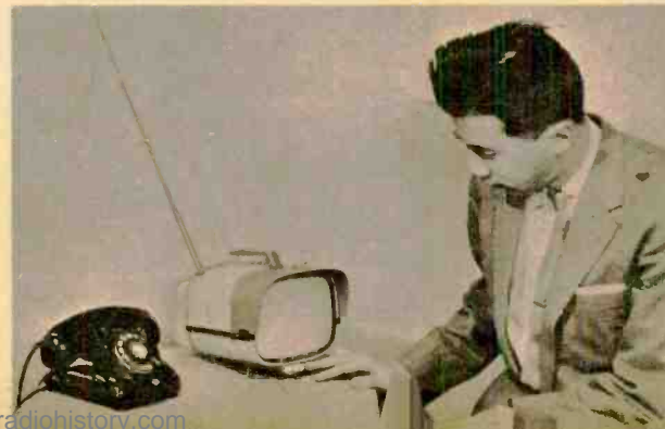
Low-cost battery is in unit that may be unplugged from set for charge. Four knobs at rear are brightness, vertical, horizontal and video gain. Below, note phone size of set.
