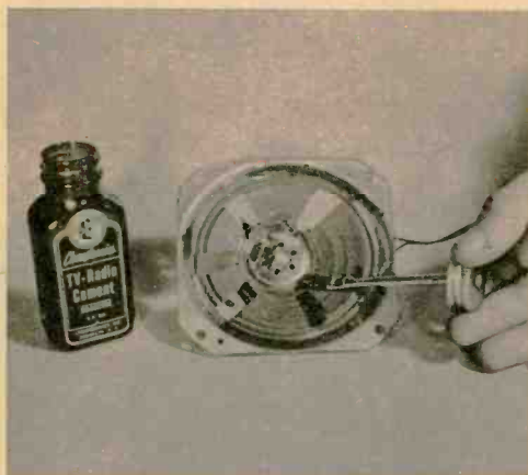
Perforated disc with solder bead sweated in center is glued over speaker voice coil.
