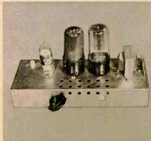
Simple AC/DC amplifier used to drive separate external speaker reproducing echo effect.
