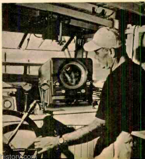
A complete radar system for the small boat is offered by Raytheon for $2195. Range is 12 mi.
