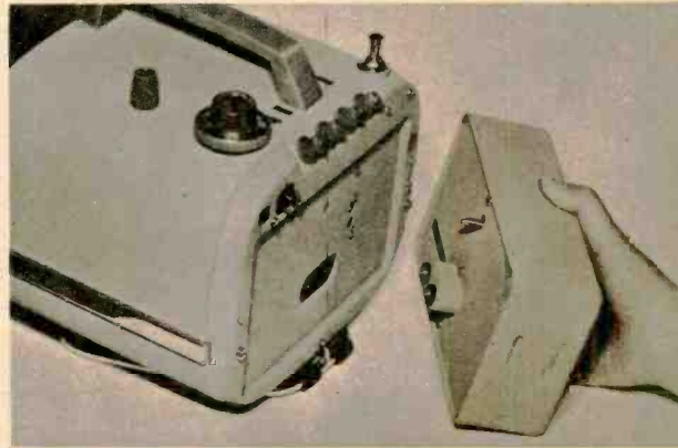
Low-cost battery is in unit that may be unplugged from set for charge. Four knobs at rear are brightness, vertical, horizontal and video gain. Below, note phone size of set.
