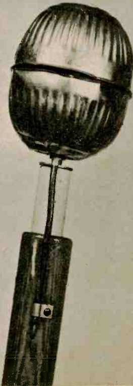
Fig. 1. Detail of Pogo's capacity ball at top of mast. Standoff insulator is porcelain type.
