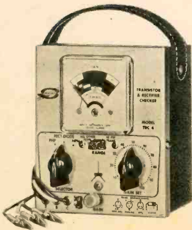
Fig. 1. Sencore varies ( R_1 ) to set 1.5 ma in collector circuit.
