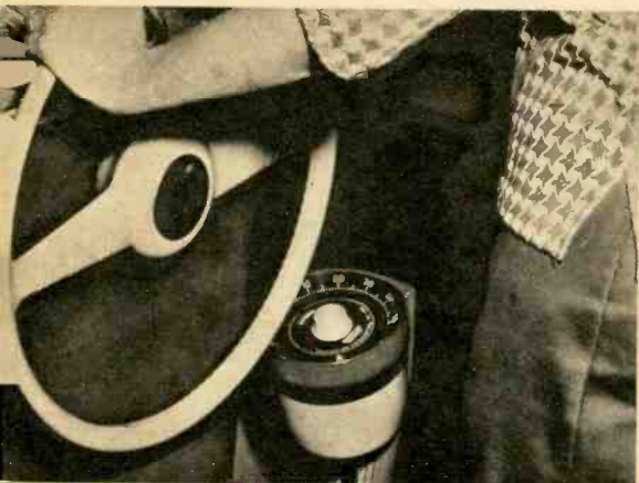
Depth indicator should be near helm in shade. Transistorized unit is Raytheon DE-708 ($125).
