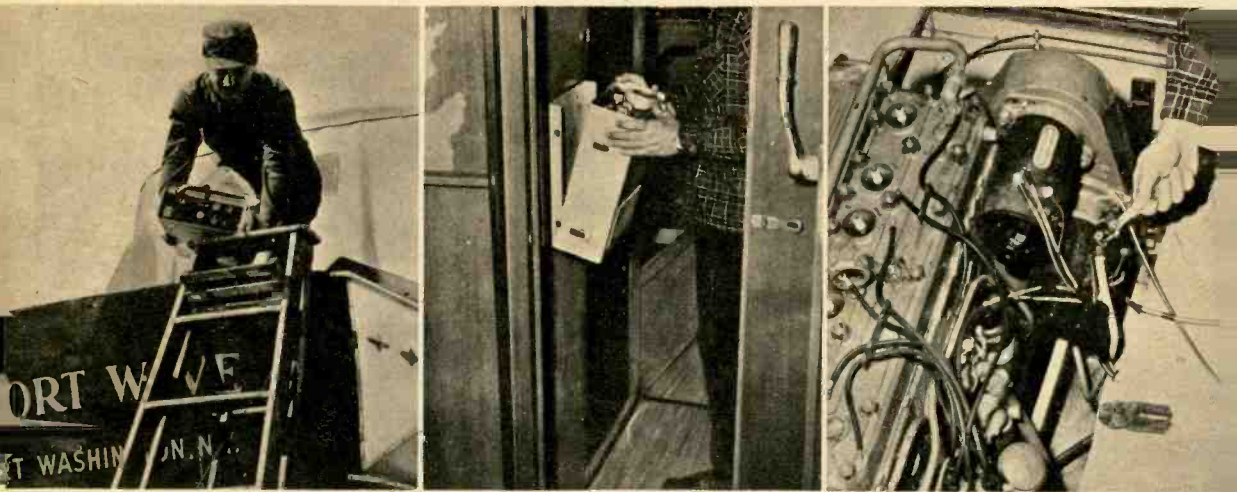
Radiotelephone goes aboard Short Wave on calm day. Careful work requires steady platform. Companionway location is protected, convenient to helm. Right, power cables are connected to starter solenoid "hot" terminal, engine block. Be wary—fireworks if you ground wrench while on hot terminal.
