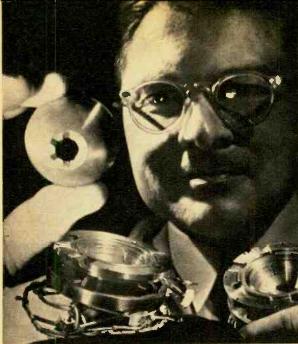
Strange behavior of some metals near absolute zero enables this super-accurate gyro sphere to be suspended solely by a magnetic field so that it can rotate rapidly in a vacuum.
