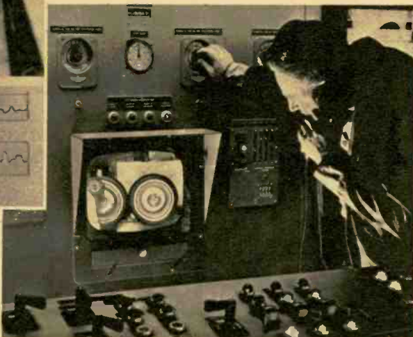
Firestone physicists record noise and vibration in road test of experimental tires. Tapes (4-channels) are analyzed and charted in lab. Polyester (see chart) gave more even ride.
