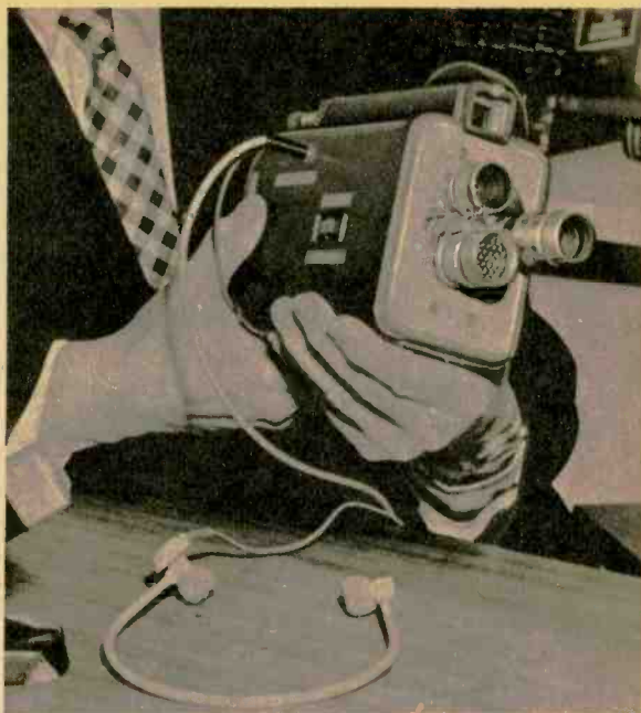
Transistorized Fairchild 8mm camera makes home movies "talkies" at time of exposure.
