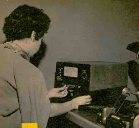
Grado-designed apparatus permanently and safely magnetizes the polished magnet metal in just 1/10,000th second with 21,000 amps, 450 volts. Magnet held without fear.
