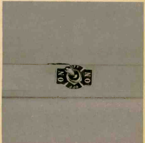
Three-position toggle switch provides control of illumination, either dim or brilliant.
