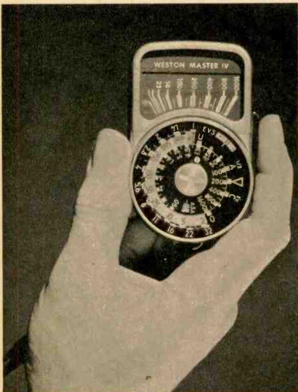
Basic, versatile exposure meters have had to keep pace with faster films, lenses and shutters. This meter handles 0-25 foot candles.
