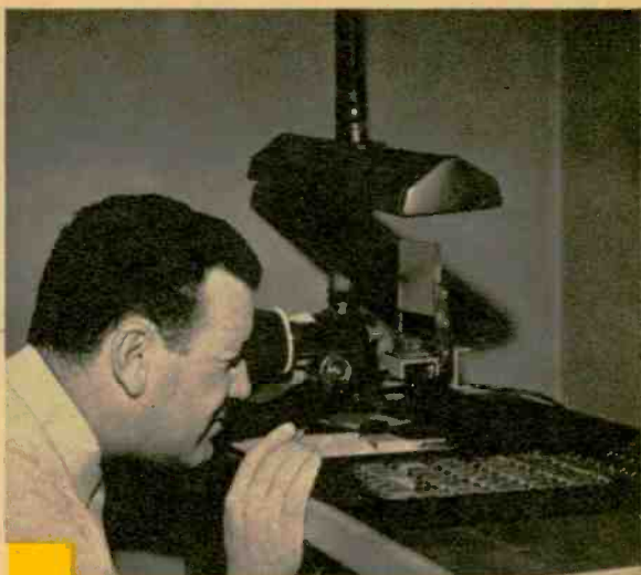
Orienting the diamond in plastic stylus arm is accomplished by sighting through cross-haired lens of horizontal microscope and applying hot tweezers to reform the plastic.
