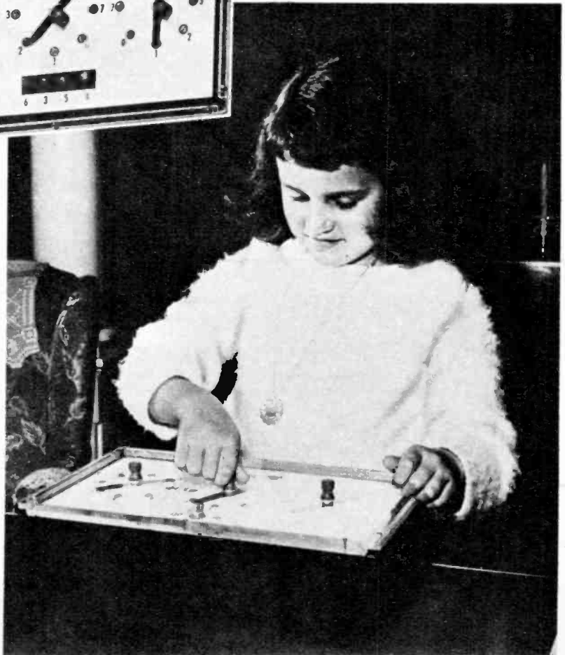
Completed unit at left is covered with a Lucite face. Three sets of numbered brass bolts provide the switch contacts. At bottom center, neon lamps are seen.
