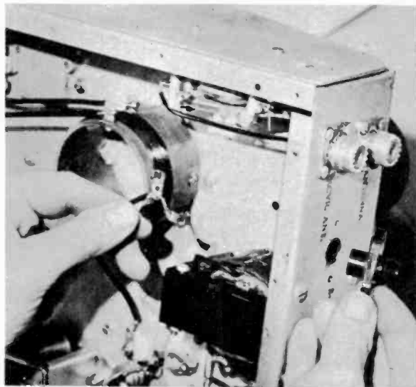
"Stop, Look and Listen." Here a high voltage bushing (right) broke down and shorted out to chassis. Traces of carbon are seen on chassis.
