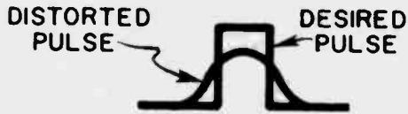
Fig. 5. Use of 'scope without low-capacity probe produces distortion of square waves.
