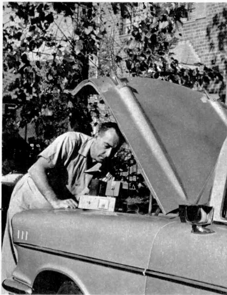
Auto radio supply in use as a car battery charger. It will supply either 6 or 12 volts.
