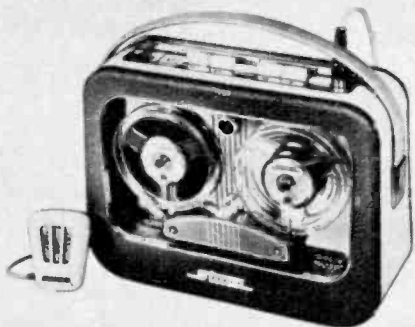
Stuzzi comes from Austria and records on two speeds. Push-button controls are on the top.
