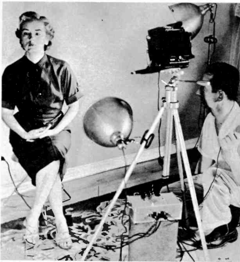
Unit is between tripod legs with two photofloods plugged into it. Photographer presses solenoid button which will turn up floods and release shutter.
