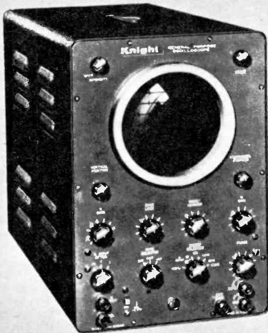
Fig. 2. Vertical input attenuator is along lower left edge of panel. Fig. 3 is at right. A vertical polarity switch will reverse the pattern.
