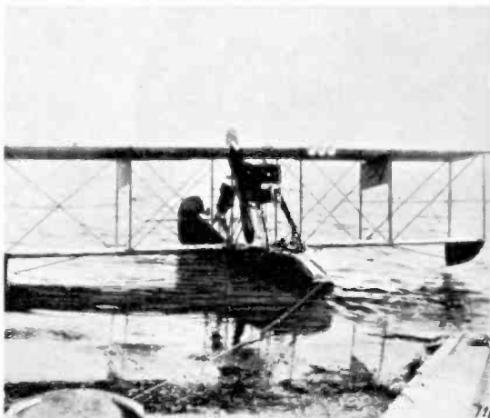
Curtiss F-boat is rigged for automatic flight. Pre-set flight plan worked, but plane was not designed to carry the required bomb load.
