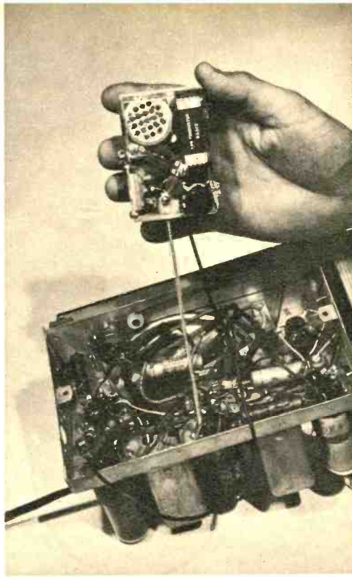
Stiff wire probe is touched to input and output stages of table model broadcast set.
