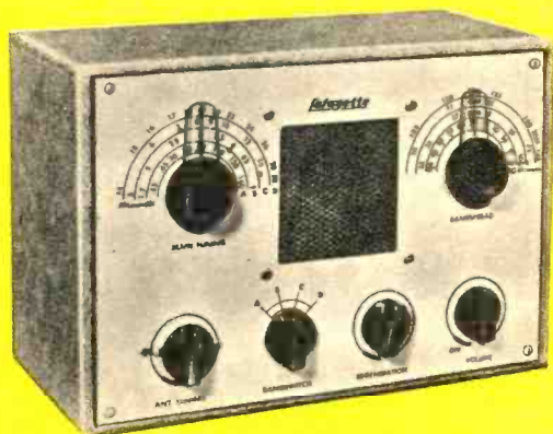
At top is the Heathkit model AR-3 4-band receiver which sells for $29.95 without the cabinet. Its tube complement numbers five, with beam power output. Amateur bands are marked off on the slide rule dial face. Below is the Lafayette 3-tube "Explor-Air" kit that can be bought for only $18.50, less case. It has features found in more expensive receivers, such as bandspread tuning.
