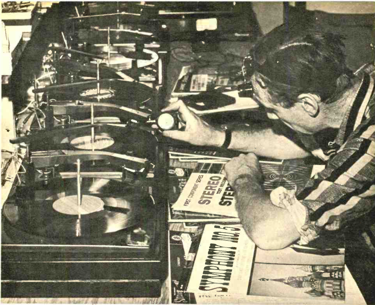
Gauge measures stylus force. Incorrect adjustment was found to produce excessive record wear.
