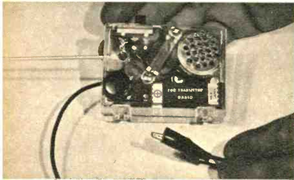
Note holes for speaker at upper right. Alligator clip goes to ground of set under test.
