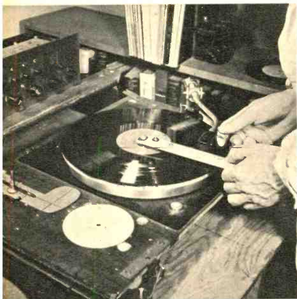
Rapid location of specific passages on record was aided by ruler pivoted on turntable post.
