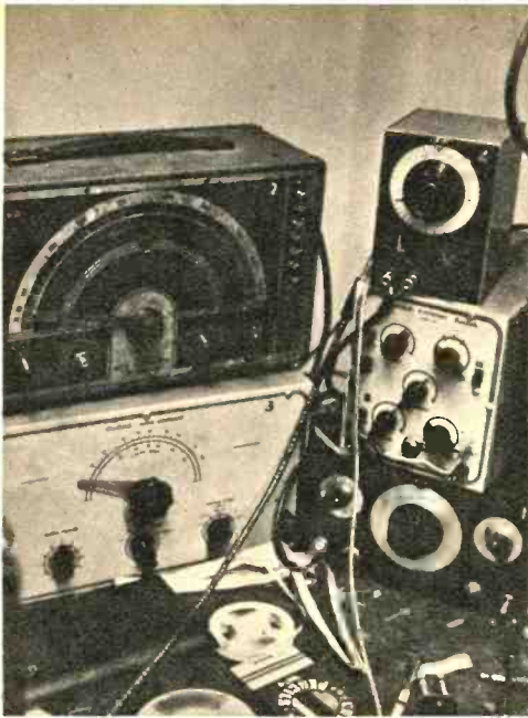
BFO, signal generator and electronic switch are used to create regular rhythmic patterns of pure tones. At right, author's "Composition for Tape Recorder" rests on desk in front of recorders, mixers, etc. Five recorders, two mikes, eight oscillators may be mixed at once.
