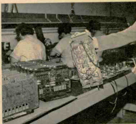
Complete circuit can be assembled at factory. Hand and dip soldering techniques are used.
