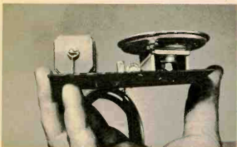
Finger points to screw used to hold speaker to board. It requires a slightly larger hole.
