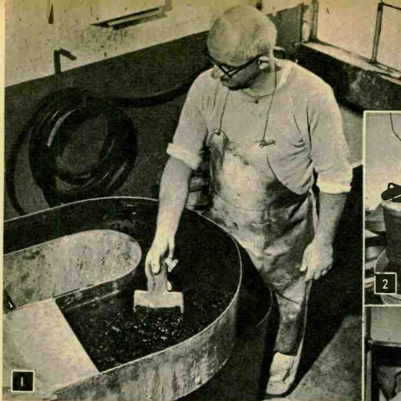
1. Making the paper mix for the speaker cones. This mix consists of water, wool fiber and pulp in carefully controlled proportions and is beaten to desired consistency in special mill.
