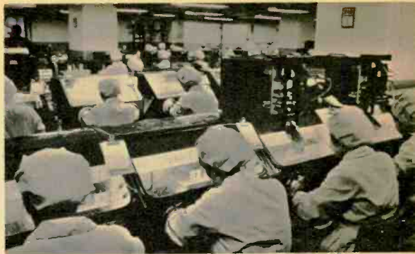
. . . other women, with their hands in special chambers, execute hermetic sealing process.
