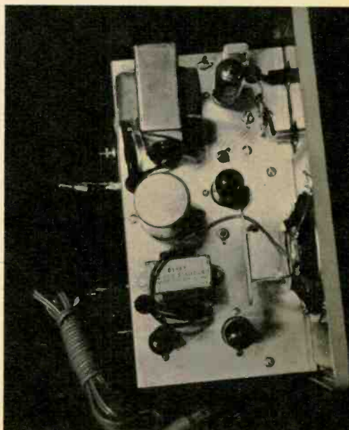
Topside view of chassis with the front panel attached. Power transformer is at upper edge.
