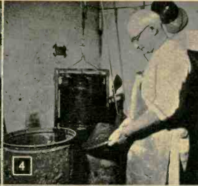
4. Cylinders are raised and cone on its form is removed from the tank.
