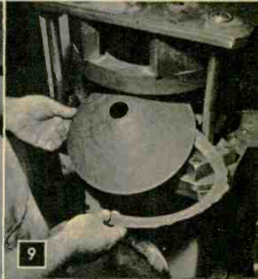
9. Die cutting press then cuts the cone to correct size; forms center hole.
