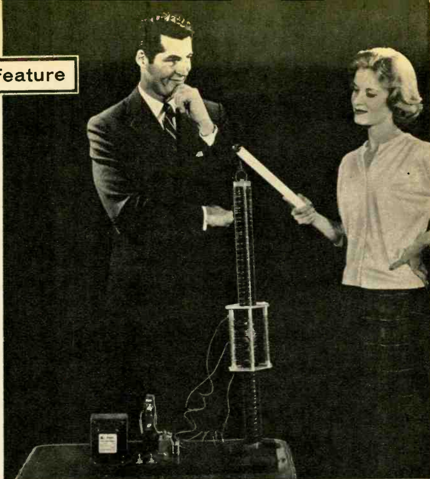
Vertical tube is secondary of Tesla coil. Wire ring on top discharges high voltage and lights fluorescent bulb. Actually, bulb lights at several feet.
