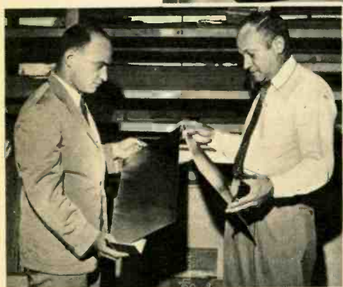
Insulating base materials may vary from paper base phenolic laminates to shock and heat resistant Fiberglas. Copper foil (other metals may be used) is bonded to one or both sides of base with tough adhesive. All raw materials are put through heat, humidity, pressure tests, above. Left, El staffer looks over uncut base stock with Photocircuits' G. Maisch (right).
