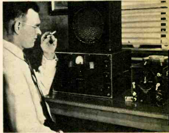
Author monitors gear that picked up Sputnik I and Lunik. Hammerlund ham set feeds signal to GE aero receiver for further amplification.
