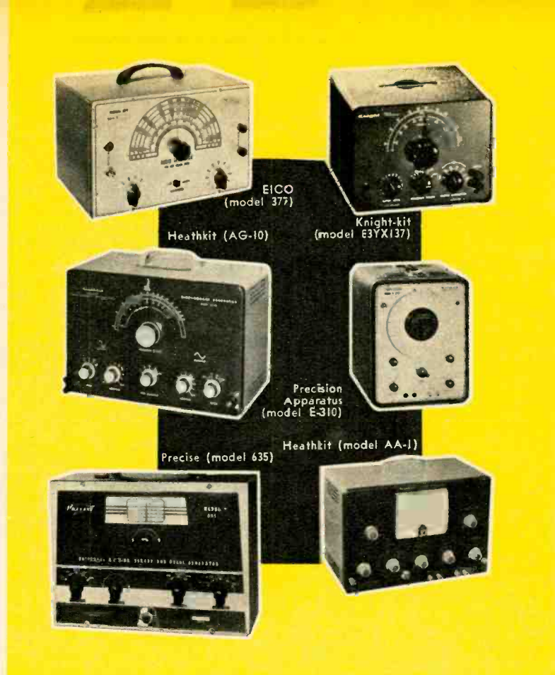
AUDIO GENERATORS: This category includes units that cover entire range of audio frequencies, and those that generate sine- and square-waveforms.
