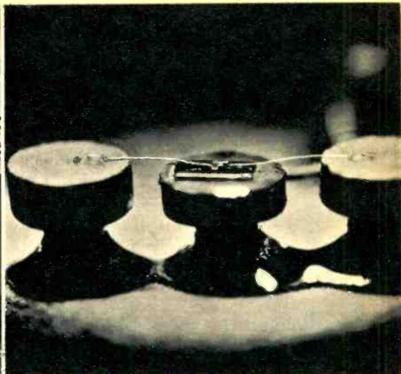
Magnified over 25 times, this photo takes you inside a diffused base germanium transistor at Bell Labs for a view of its internal structure.
