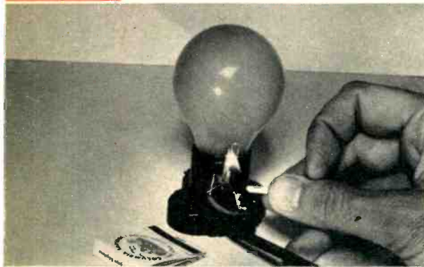
"Magic Lamp" project and its schematic. A match flame applied to the bi-metal turns the lamp on; a puff of breath blows it out. Starter is used in normally-open condition.
