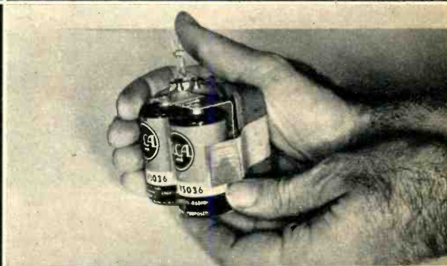
Buzzer, bi-metal electrodes, and batteries comprise a fire alarm unit. Note in schematic that many bi-metals may be wired in parallel, each for a different location.
