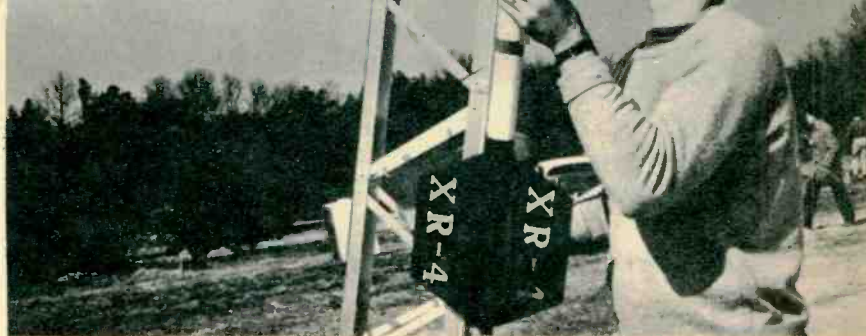
Lou Taylor, of New York City, checks for wobble and friction by moving his rocket, the XR-4, up and down specially constructed launcher and rail. This rocket sports fins somewhat larger than those of most other missiles.
