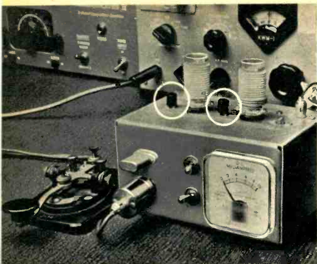
This transmitter, using only 1/10 watt and two RCA "drift" transistors, beamed a message from California to South Africa on 15 meters.
