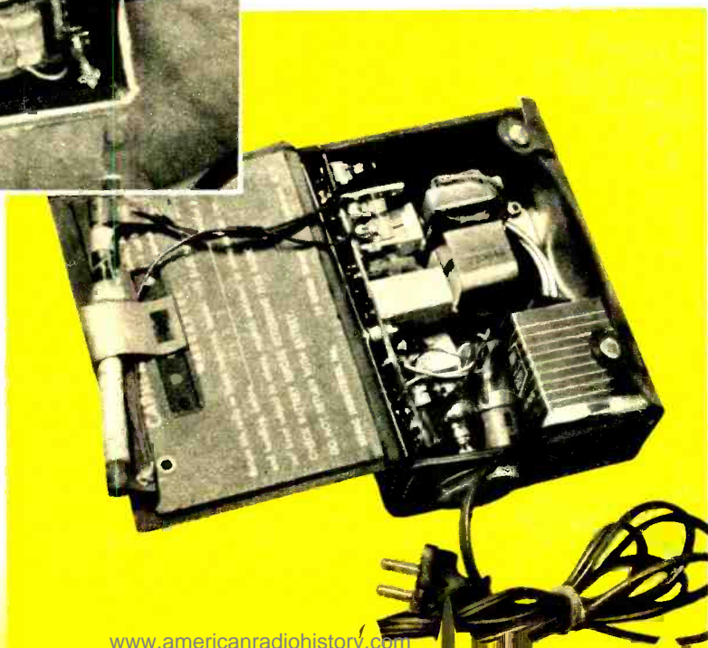
Power supply, lower right, appears like the original dry cell, except for AC line cord.
