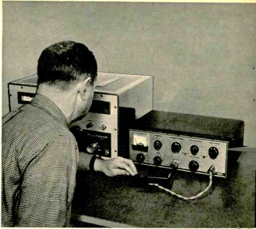
The transmitter is compact with low silhouette. The crystal socket is at bottom of panel. Meter is calibrated for 75 watt Novice operation.
