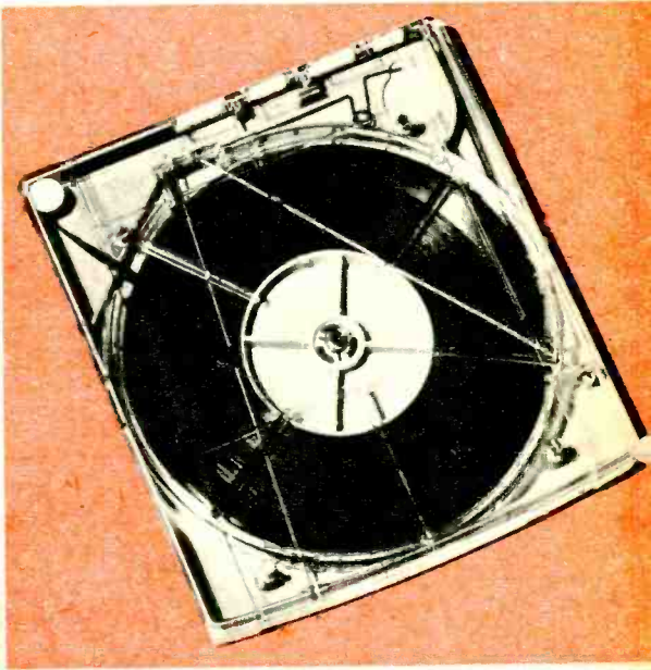
No flipping with this tape magazine. One-spool design and Mobius loop permit continuous play.
