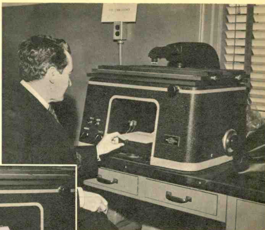
Densitometer is used here to compare spectral lines of two samples. Spectral photo of known element is inserted at top of instrument where it is scanned electronically, then projected for comparison with photo of doubtful element.
