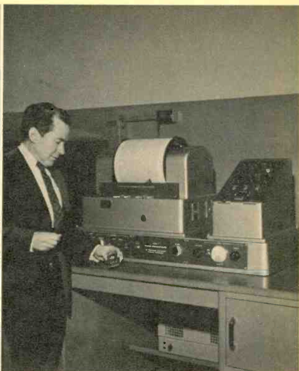
Narcotics sample, held between salt slabs, will be fitted to infrared spectrophotometer.
