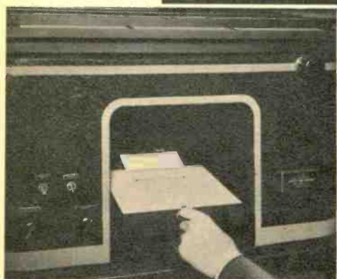
Densitometer is used here to compare spectral lines of two samples. Spectral photo of known element is inserted at top of instrument where it is scanned electronically, then projected for comparison with photo of doubtful element.
