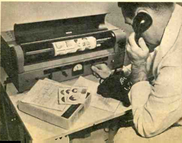
Fingerprints of criminals, along with "mug shots" and records may be transmitted rapidly to police agencies all over the country by speedphoto equipment, which is similar in operation to facsimile.
