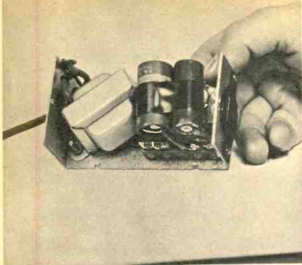
Power supply chassis. Visible from left to right are 117 volt line cord, T, C6, C7, and SO2.
