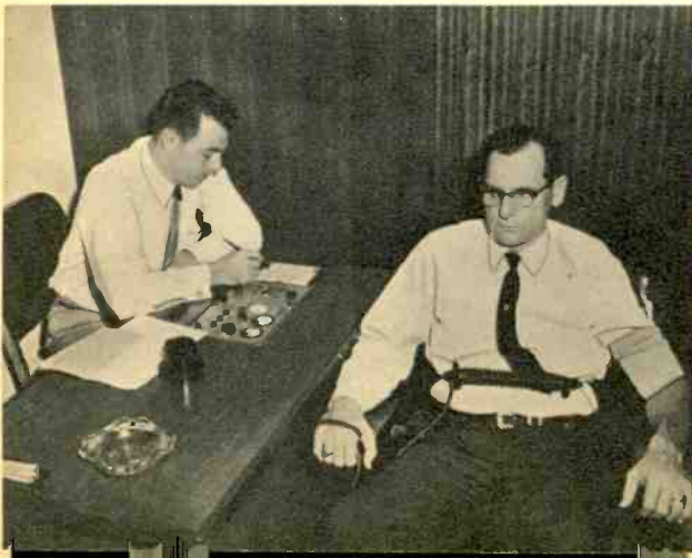
Keeler polygraph, often called the "lie detector," is demonstrated by Texas Department of Public Safety experts. The instrument records physiological changes in suspect during planned questioning period.
