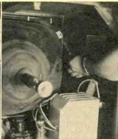
10. The nuts are removed from the 4 studs that secure the forward part of the tube.
