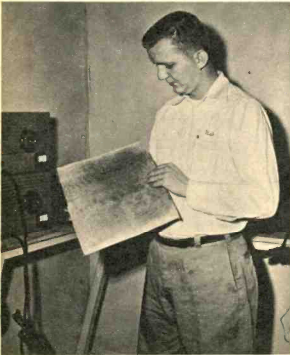
Willier method of recovering silver from photographic hypo uses wire mesh electrode.
