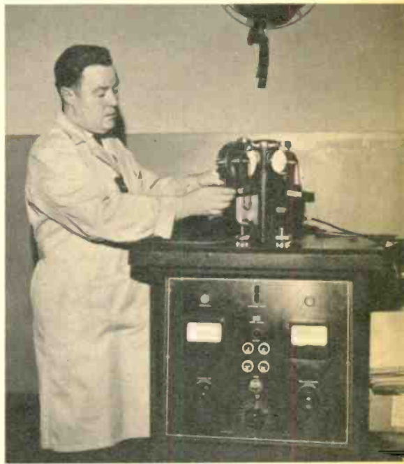
Right, Detective Kevin O'Brien adjusts cylindrical X-ray diffraction camera. Inside the non-optical camera is a confiscated sample of heroin hydrochloride. Film, left, shows concentric arcs formed by diffracted X-rays. Measurements can be made to classify sample, which is not destroyed.
