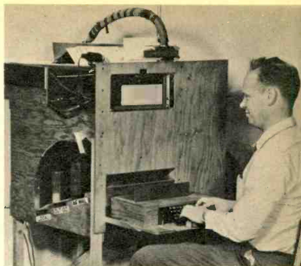
Prototype mail sorter allows operator to send letter into one of only three mail groupings.
