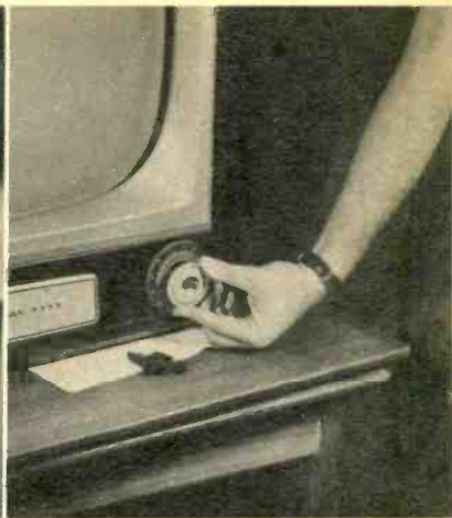
11. If tube is obstructed, chassis must be moved out of the way. Pull off knobs.
