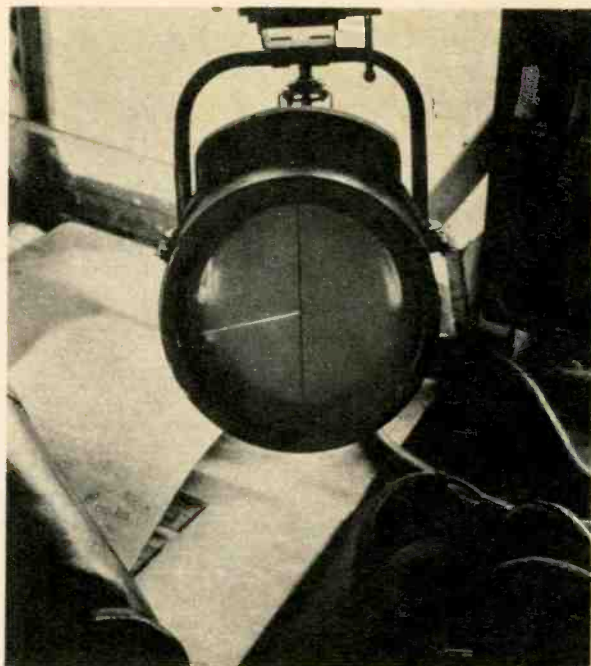
Any object on the ocean's surface will appear as a white pip on this Surface Radar Scope.
