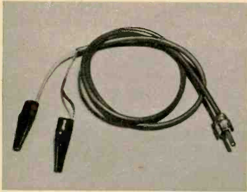
Accessory cable has insulated alligator clips on one end, with plug for jack J2 on the other.
