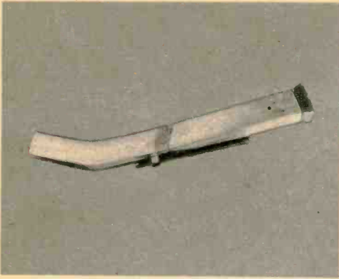
Top view of arm. Counterweight to the right is a chunk of lead filed to shape. The thin brass rod is for adjusting stylus pressure.
