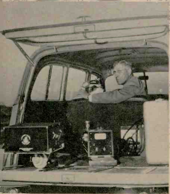
Radar gear transmits signal which bounces off passing car with changed wavelength
