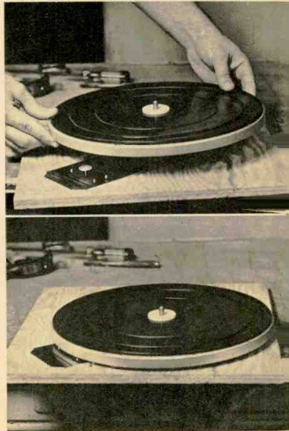
The light aluminum turntable with its rubber "Discushion" is lowered onto spindle. With the addition of pickup arm, base, and switch, the unit is complete. Turntable speed is 33\frac{1}{3} RPM.
