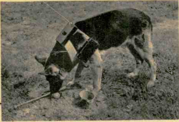
Aruk finds child's toys and growls. This is picked up by throat mike, sent out to master.
