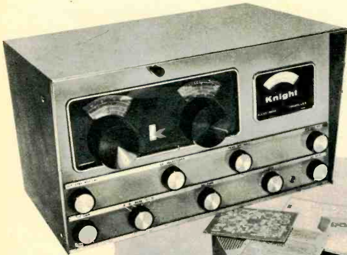
The assembled Knight kit receiver with "S" meter is shown at left. First spread out all parts as shown to identify and check them against the parts list in the manual.
