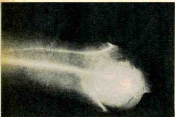
Actual photo of high-energy pinched gas (central track) rounding a curve in Perhapsatron.
