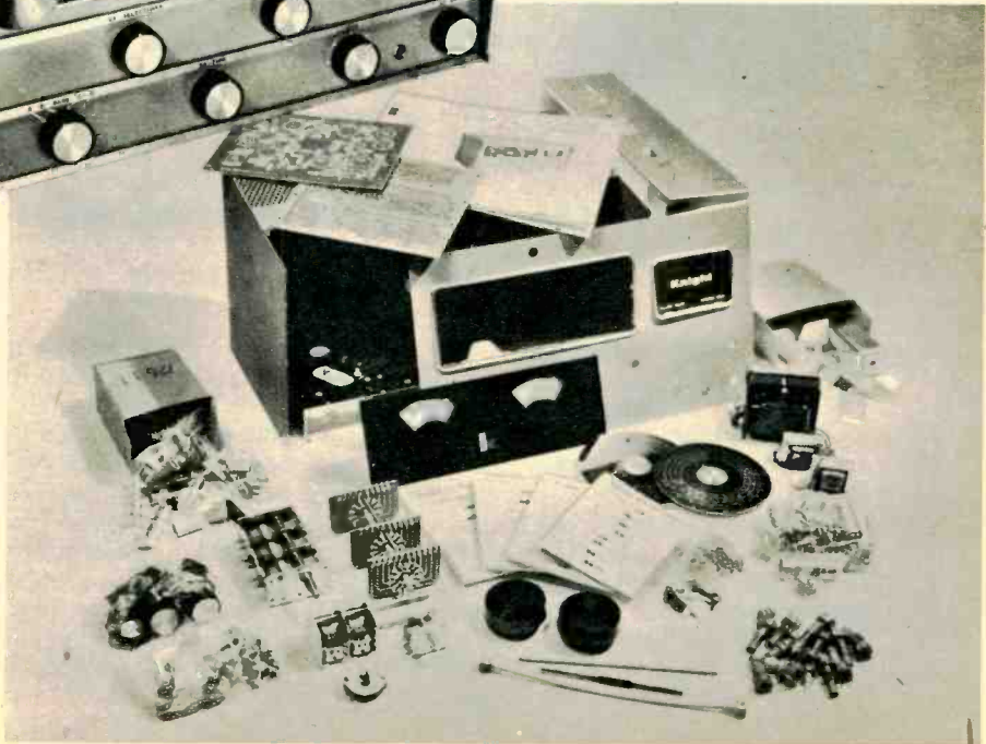
The assembled Knight kit receiver with "S" meter is shown at left. First spread out all parts as shown to identify and check them against the parts list in the manual.
