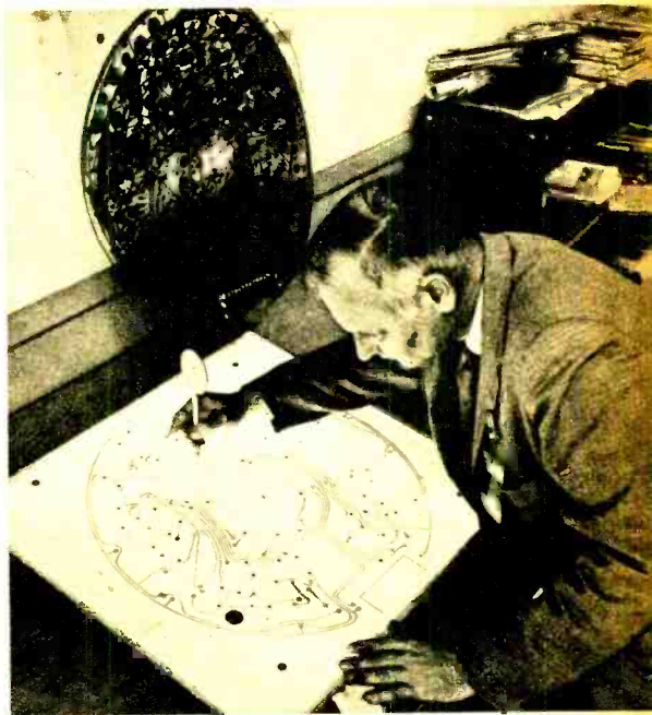
Tracing a printed circuit is a first step in preparing a transmitter to be used in a satellite.
