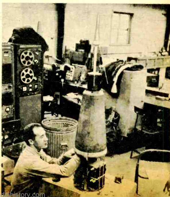
Magnetic field measurements in the ionosphere are carried out with this instrument in rocket.
