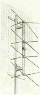
Figure 2. Pictured here is the stacked bow-tie with reflecting screen with alternating hot and dead spots.
