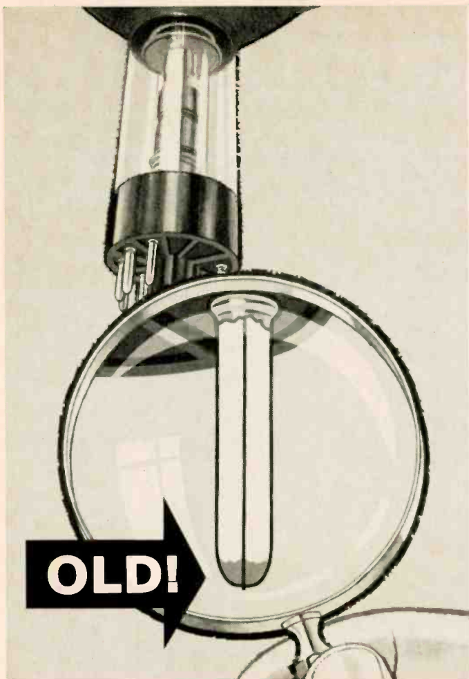
The "old" conventional pin soldering method relied upon contact between pin and wire only at their tips.
