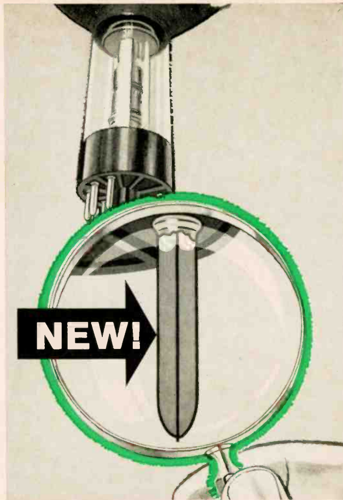
New Sylvania pin soldering technique extends solder far up into the pins—provides maximum contact with the wire—assures low electrical resistance and high mechanical strength.
