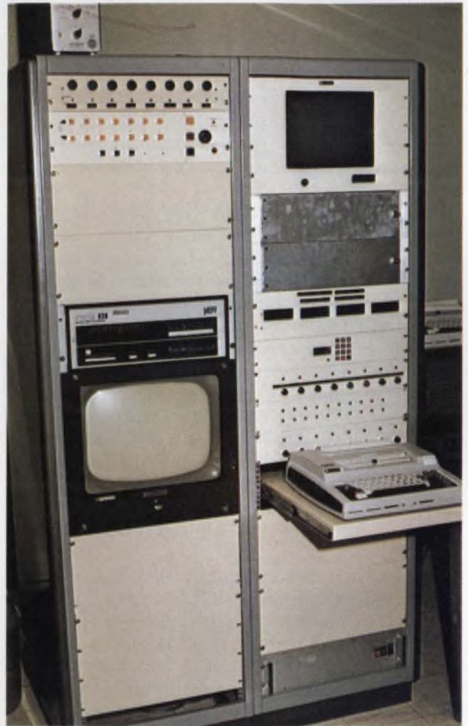
These 8080 microcomputers incorporated at NASA test sites change system architecture by centralizing, not distributing, the minicomputers the 8080s feed.
