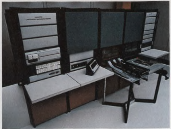
Testing \mu P boards is a challenge, and the answer comes from automatic test systems like this Teradyne L135. Price starts at a mere $150,000.
