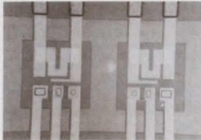
Two transistors can hang in space thanks to a controlled etching process. The IC is only 3 mils thick.
