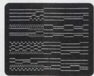
Time Domain. Timing diagram lets you see the sequential and simultaneous relationship between digital signals, to simplify hardware troubleshooting.
