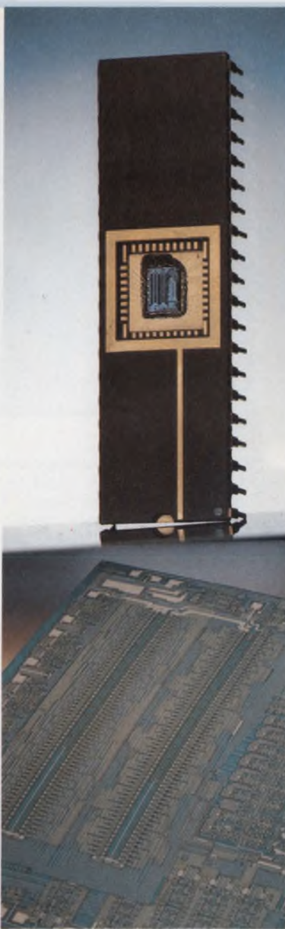
First of its kind: This single-chip data-acquisition system includes an 8-bit a/d with Tri-state outputs, a 16-channel multiplexer and logic control to interface \mu Ps (National).
