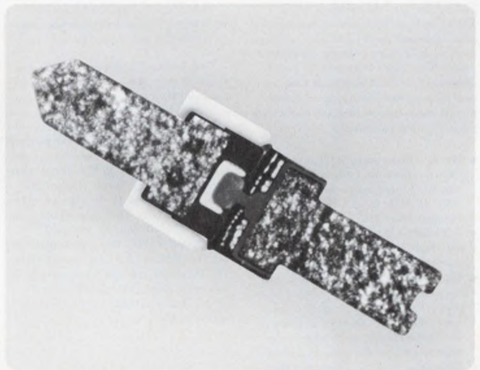
The HP mesa process with glass backfilling is responsible for the performance of this beam lead PIN. The mesa construction constrains the minority carriers, thereby enhancing switching speed.
