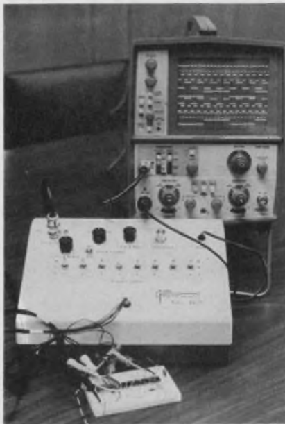
Eight lines in timing-diagram format can be displayed on a scope screen with the Kenmark Model RK778—which goes for just $225.
