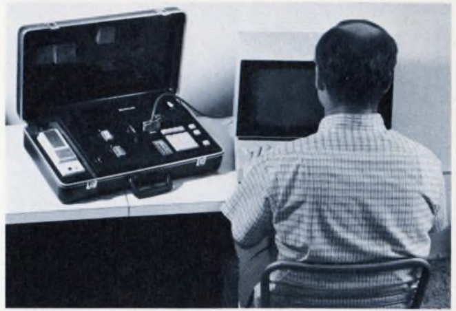
With an RS-232 interface, the series 90 PROM programmer from Pro-Log lets you enter programs from a CRT terminal directly into the PROM to be programmed or into an optional RAM workspace.
