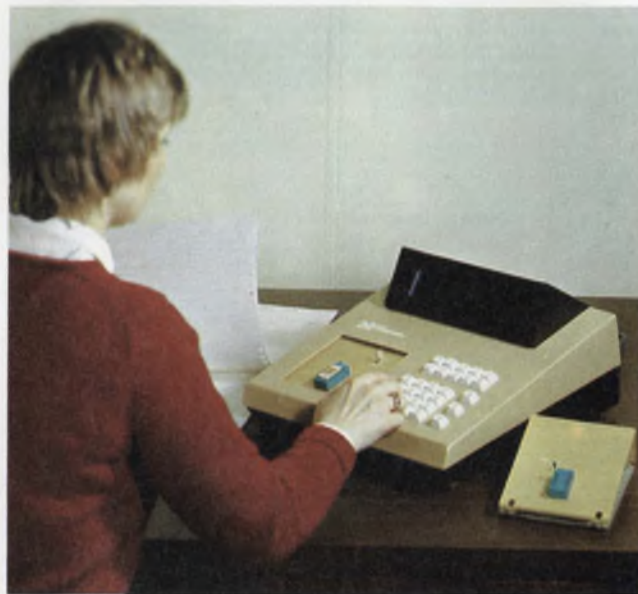
Able to program any bipolar or MOS PROM, the IM1000 programmer from International Microsystems includes a TTY interface as well as two RS-232 ports as standard.
