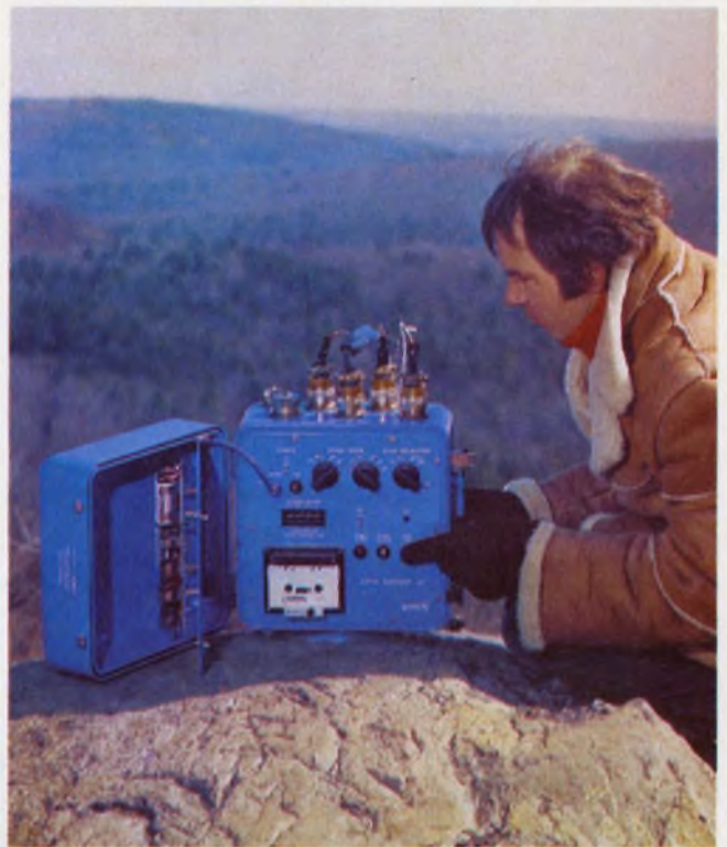
Data-Logger-2 can record 64 analog channels as a string of 14-bit words. This battery-powered, cassette, weather-proof data-acquisition and recording system, from Datel, can run for up to a year on one charge.
