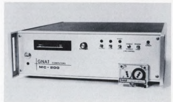
Hardware and software control 3M's DCD-100 mini-cartridge drive in Gnat Computers' \mu P-based MC-200.
