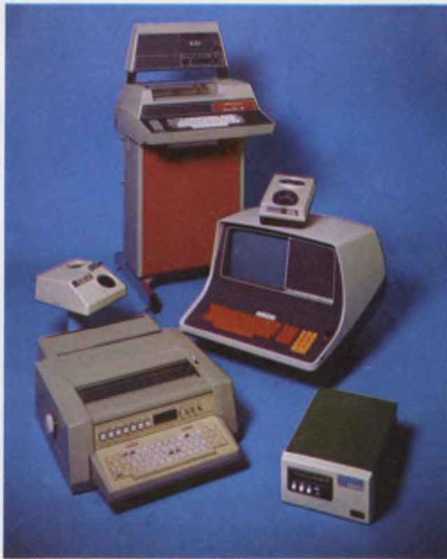
Data-communications equipment includes (clockwise from top) General Electric Terminet 30 teleprinter, which gives hard copy; Livermore acoustic coupler, which brings a telephone handset to computers; ADDS CRT terminal, which gives soft copy; Vadic VA3400 full-duplex modem (MOdulator-DEModulator), which operates at 1200 bits/s; and the Terminet 300 and acoustic coupler.
