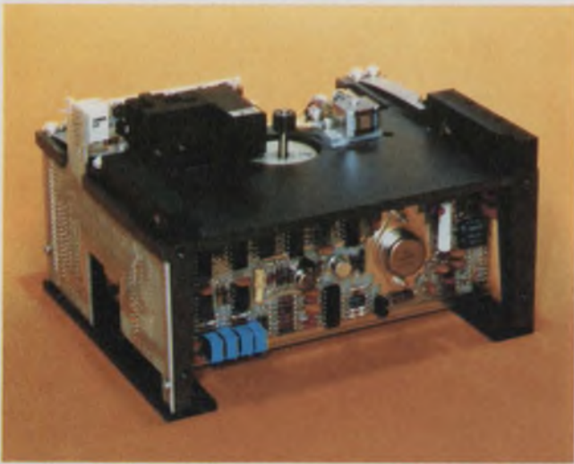
The 3000-S2 drive meets ANSI standards for processing data on X3B5/75-43 type cartridges. The Data Electronics unit reads and records per standards X3B5/75-44 (serial) and X3B5/75-53 (parallel).
