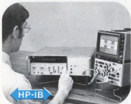
The HP 5345A super performance counter can accurately measure short RF pulses or rapidly swept signals.
