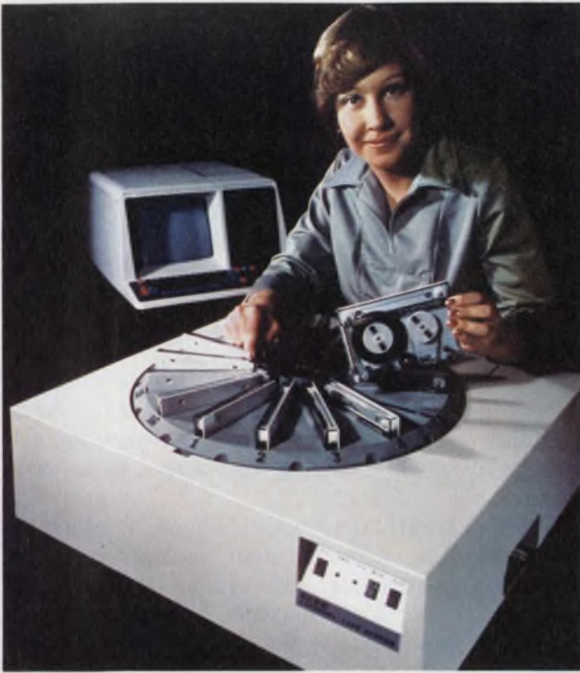
A 32-Mbyte capacity is featured in the 5200 carousel-handling and drive system , in which 16 cartridges can be accessed four at a time. The National Computer Systems unit meets ANSI X3.56-1976.
