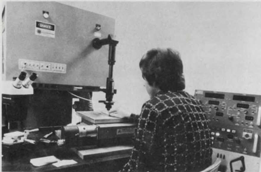
Prototype of Coherent Radiation's Everlase 150S shows the system elements: Laser (in cabinet, top left) delivers beam through the black tube to the numerically controlled work table. Controller is at right.
