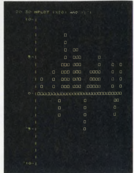
Simple instructions can specify graphic display (above, bar chart) of interactive computing results.
