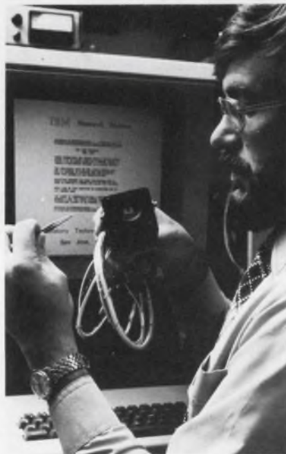
Gallium arsenide laser (in tweezers) mounts on heat sink inside laser module for IBM's liquid-crystal projection display system.
